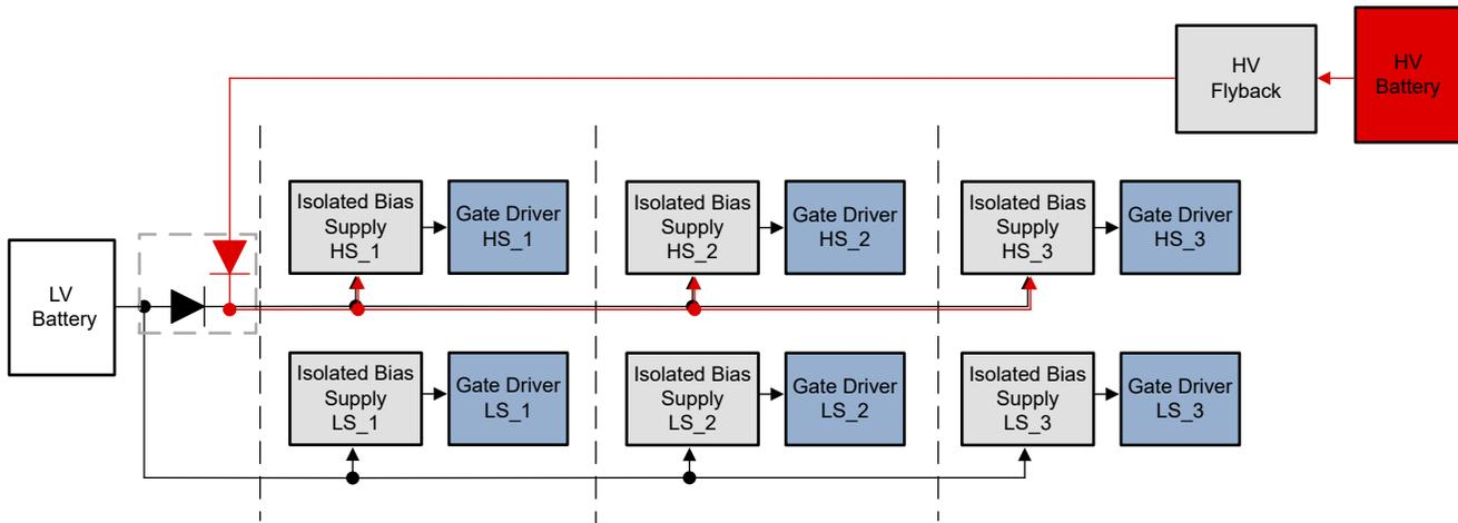
**Figure 6-4. Redundancy Only at the High Side in Fully-Distributed Architecture**
