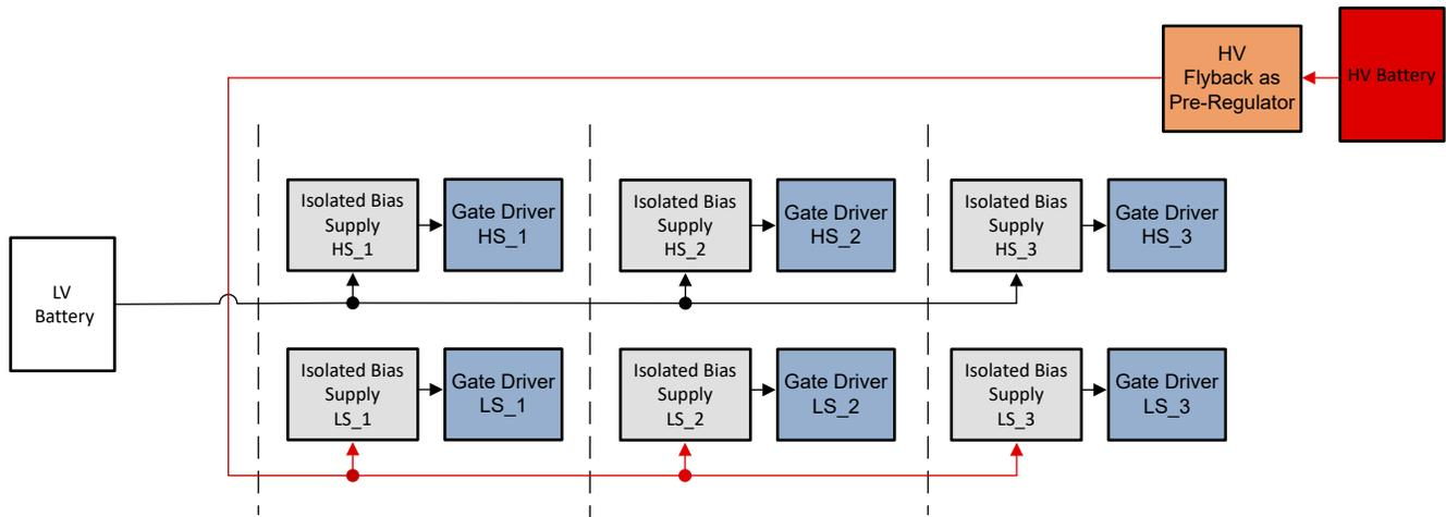
Figure 2-3. Pre-Regulator at High-Voltage Battery
