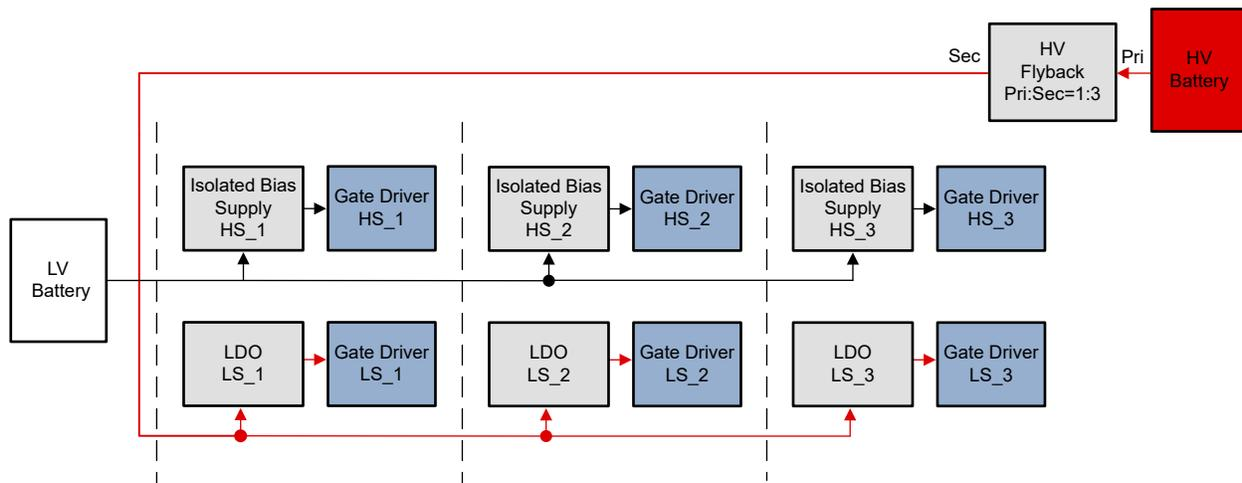
Figure 6-1. No Redundancy While Using LV and HV Batteries
