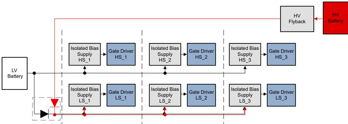
Figure 6-3. Redundancy Only at the Low Side in Fully-Distributed Architecture
