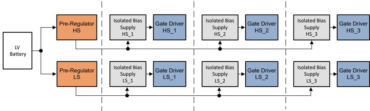
Figure 2-2. Two Pre-Regulators in a Fully-Distributed Architecture
