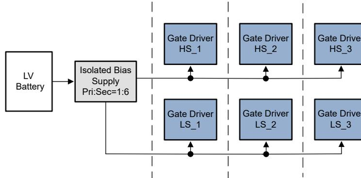
Figure 5-1. Centralized Architecture
