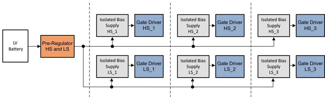
**Figure 2-1. Single Pre-Regulator in a Fully-Distributed Architecture**
