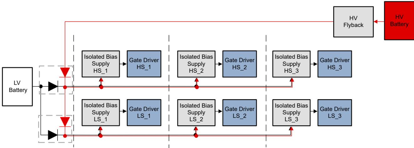
Figure 6-2. Redundancy to the all Devices in Fully-Distributed Architecture
