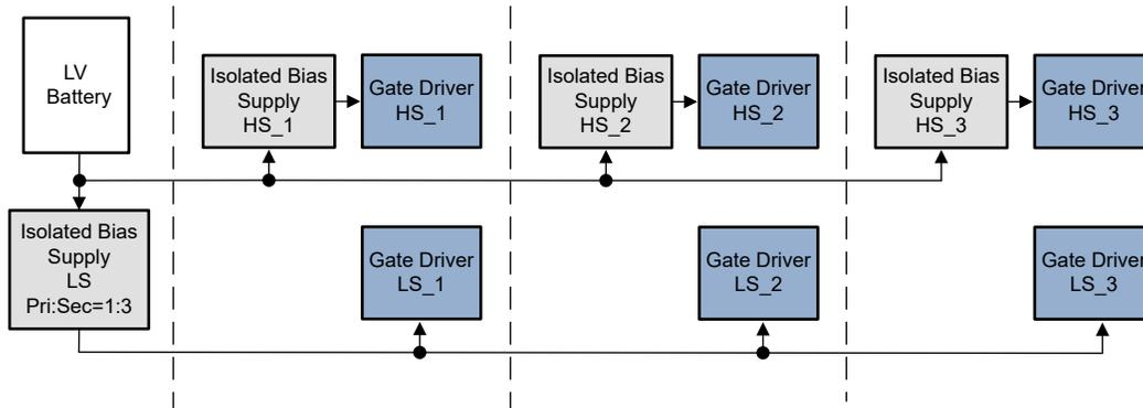
Figure 4-1. Semi-Distributed Architecture at Low Side Only
