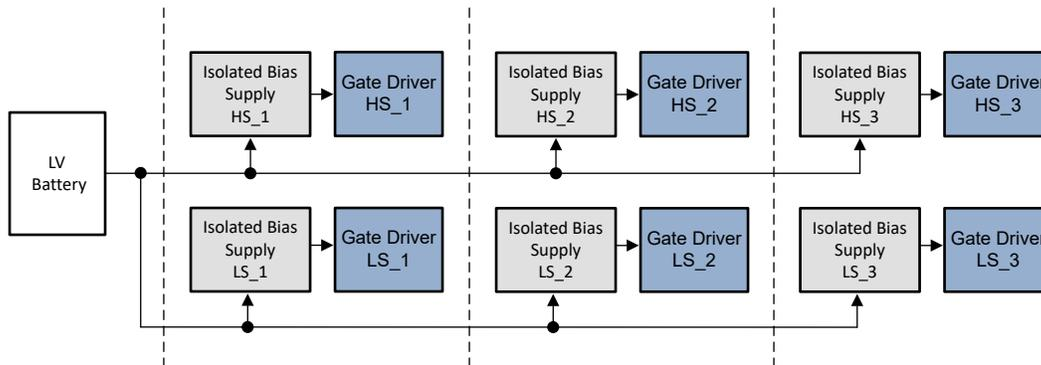
**Figure 3-1. Fully-Distributed Architecture**
