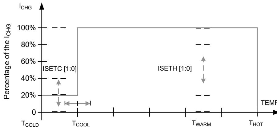
Figure 4-1. BQ25798 Charging Current Temperature Profile
