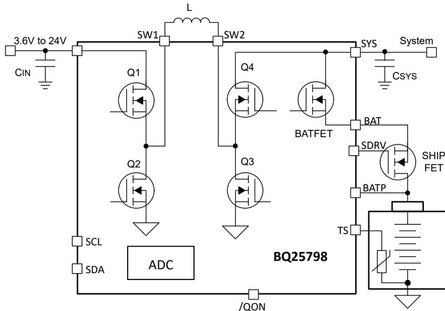
Figure 3-3. BQ25798 Fully Integrated Buck-Boost Charger
