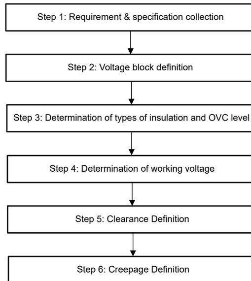
**Figure 2-1. Insulation Distance Determining Process**
