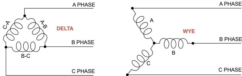
**Figure 1-5. Delta and WYE Type of Power Source**
