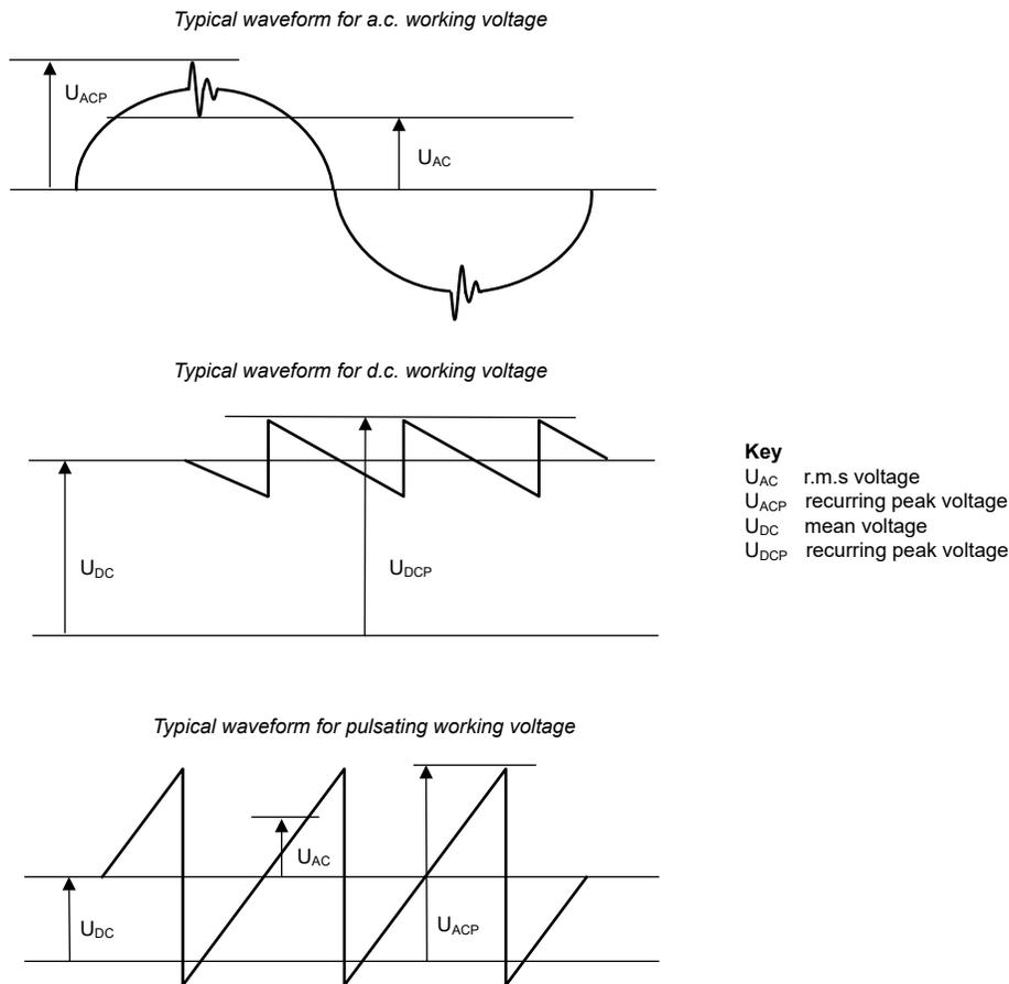
**Figure 1-6. Circuit Evaluation for Working Voltage**
