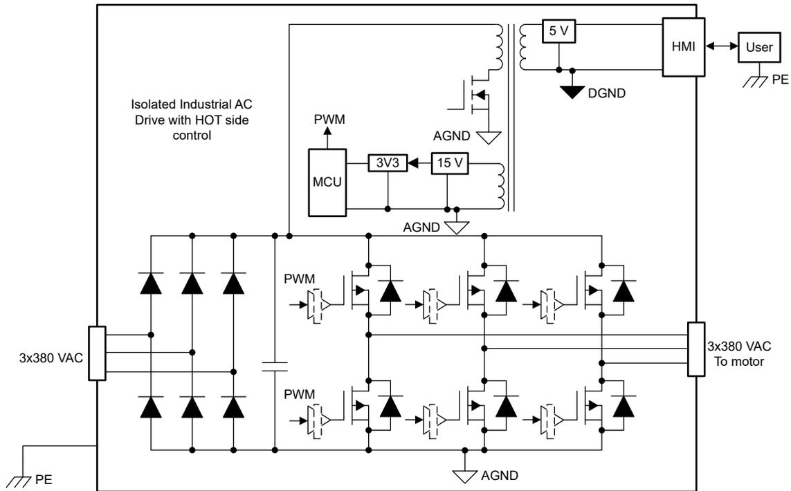
**Figure 2-2. Isolated Industrial Motor Drive System Typical Block Diagram**
