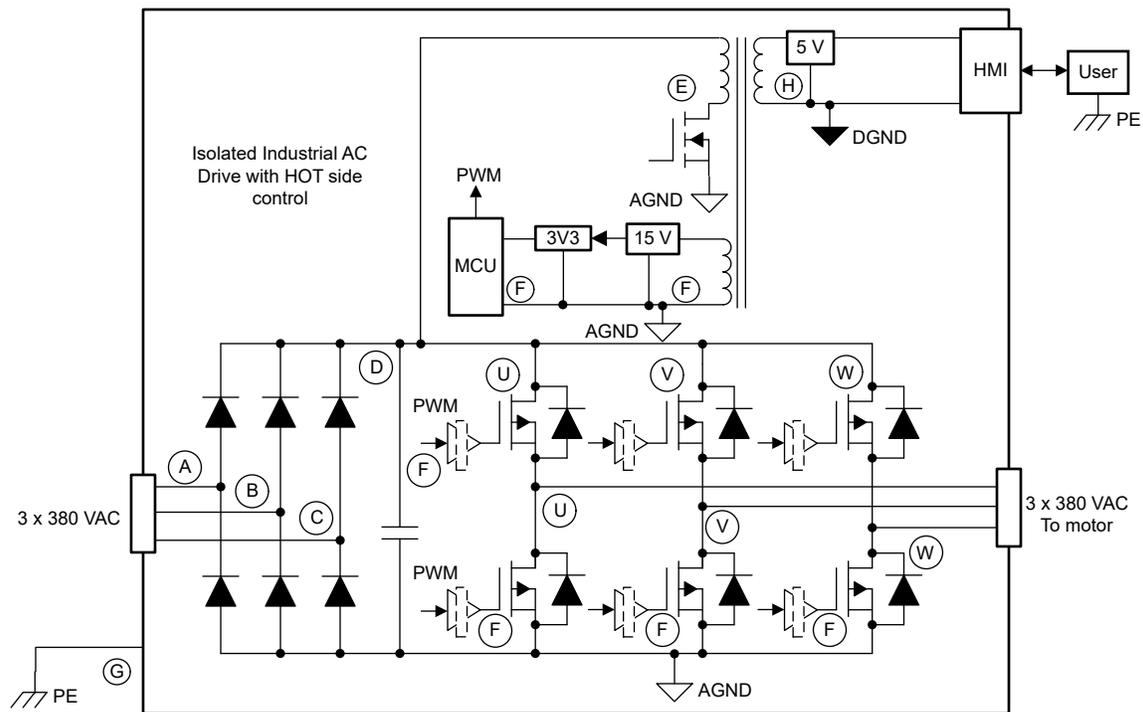
**Figure 2-3. Isolated Industrial Motor Drive System Typical Voltage Blocks**
