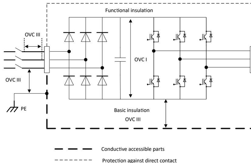
**Figure 1-4. OVC Level With Electrical Circuit Connected Directly to the Supply Mains**
