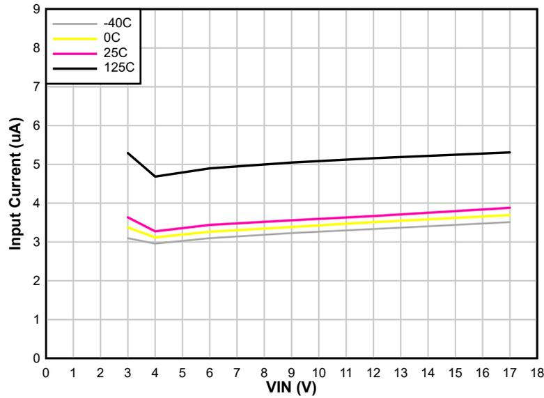
**Figure 4. Typical Quiescent Current vs VIN for TPSM82903**
