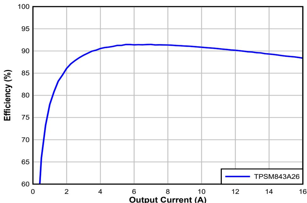
**Figure 1. Efficiency Graph TPSM843 A26 in 1.8 Vout, 12 Vin, Fsw = 1 MHz**
