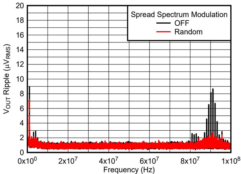
Figure 3.  $V_{OUT}$  Ripple FFT After the Second L-C Filter for TPSM82913
