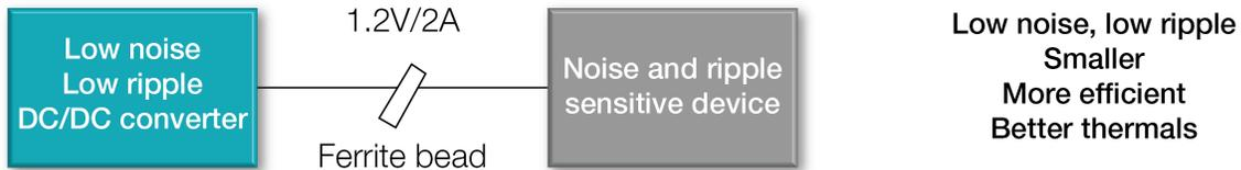
Figure 2. Example of a Noise sensitive system using a low noise and low ripple DC/DC converter
