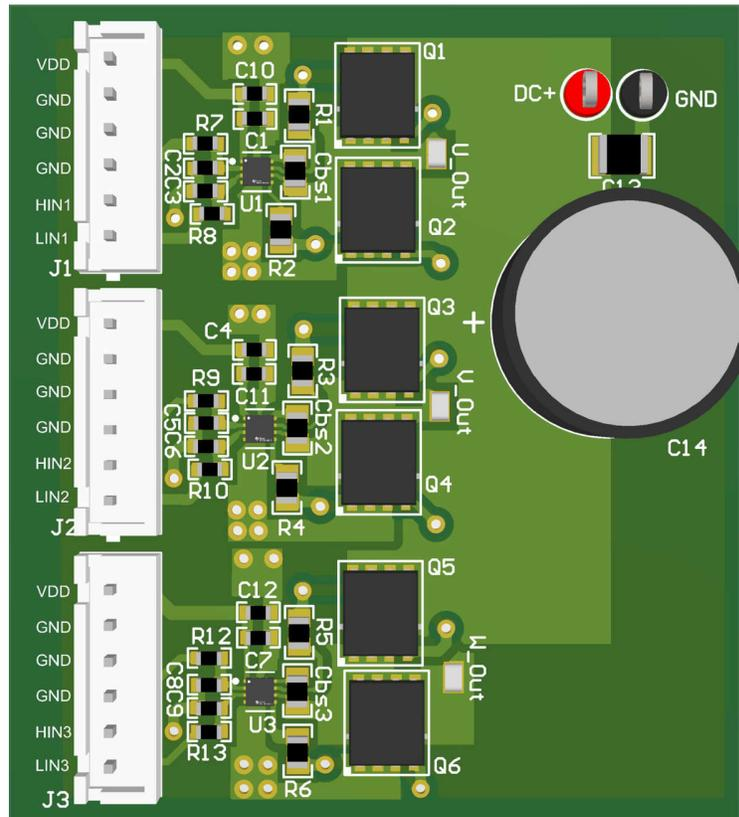
**Figure 5-1. A BLDC Motor Drive PCB Layout Example Using Three LM2105DSGR Half-Bridge Drivers.**
