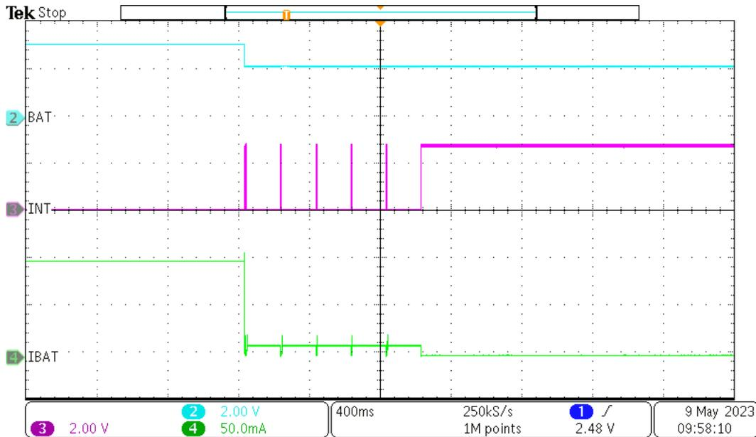
**Figure 2-3. Shorted Battery Simulation**
