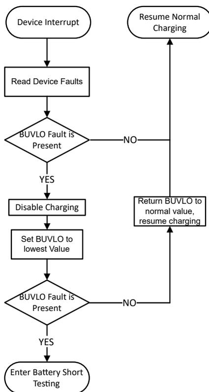
**Figure 2-1. Battery Monitoring Flow**
