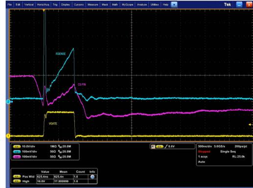
CS signal starts below 0 V, slope of CS does not follow Rsense
