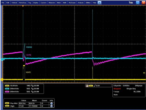
Inconsistent gate pulse widths
