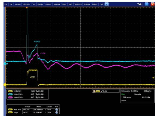
CS signal starts at 0 V, slope of the CS follows Rsense
