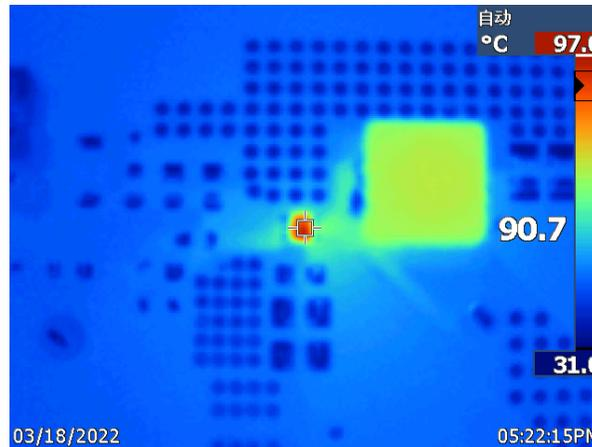
Figure 4-3. TPS566242 12-V Vin to 5-V Vout at 6-A
