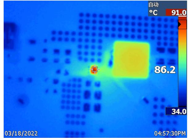
Figure 4-2. TPS566242 12-V Vin to 3.3-V Vout AT 6-A
