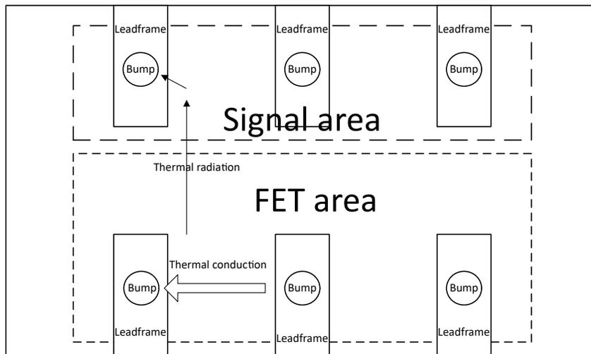
Figure 3-1. Thermal Transfer Direction
