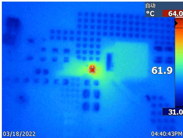
**Figure 4-7. TPS564242 12-V Vin to 1.05-V Vout at 4-A**
