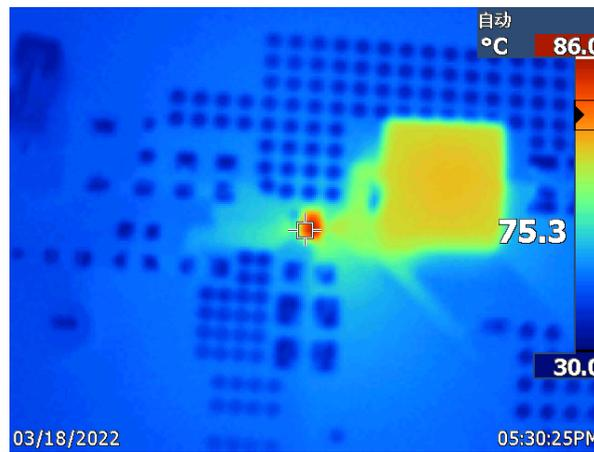
**Figure 4-6. TPS565242 12-V Vin to 5-V Vout at 5-A**
