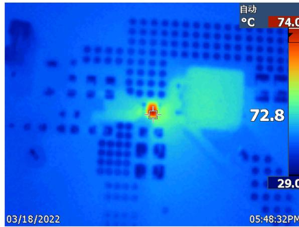
Figure 4-9. TPS564242 12-V Vin to 5-V Vout at 4-A
