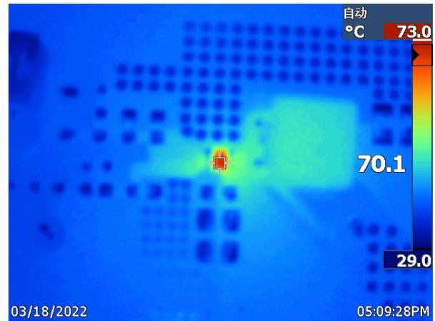
**Figure 4-8. TPS564242 12-V Vin to 3.3-V Vout at 4-A**
