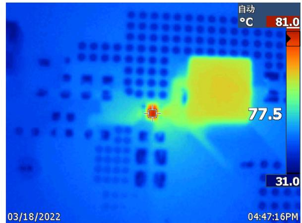
**Figure 4-5. TPS565242 12-V Vin to 3.3-V Vout at 5-A**
