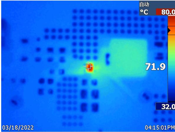
Figure 4-1. TPS566242 12-V Vin to 1.05-V Vout at 6-A
