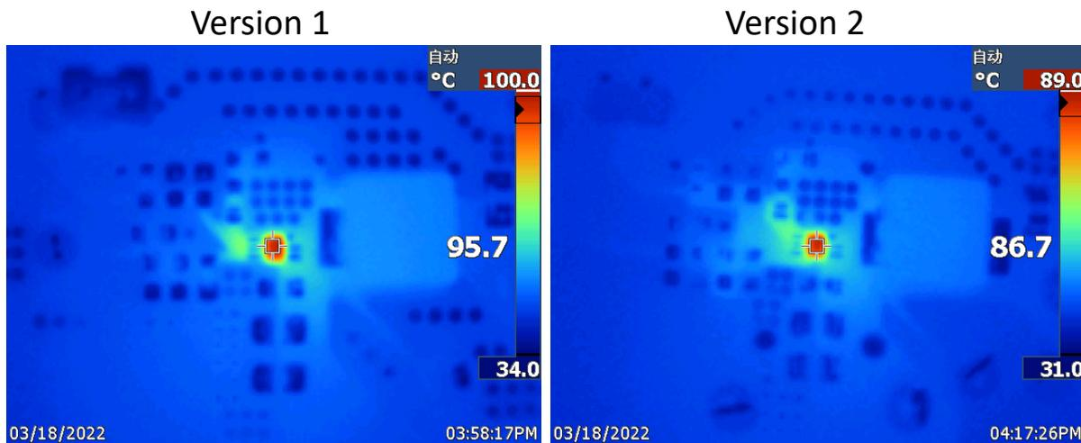
Figure 3-4. Thermal Test Result with Two Versions
