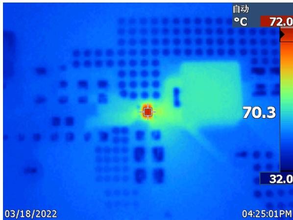
**Figure 4-4. TPS565242 12-V Vin to 1.05-V Vout at 5-A**
