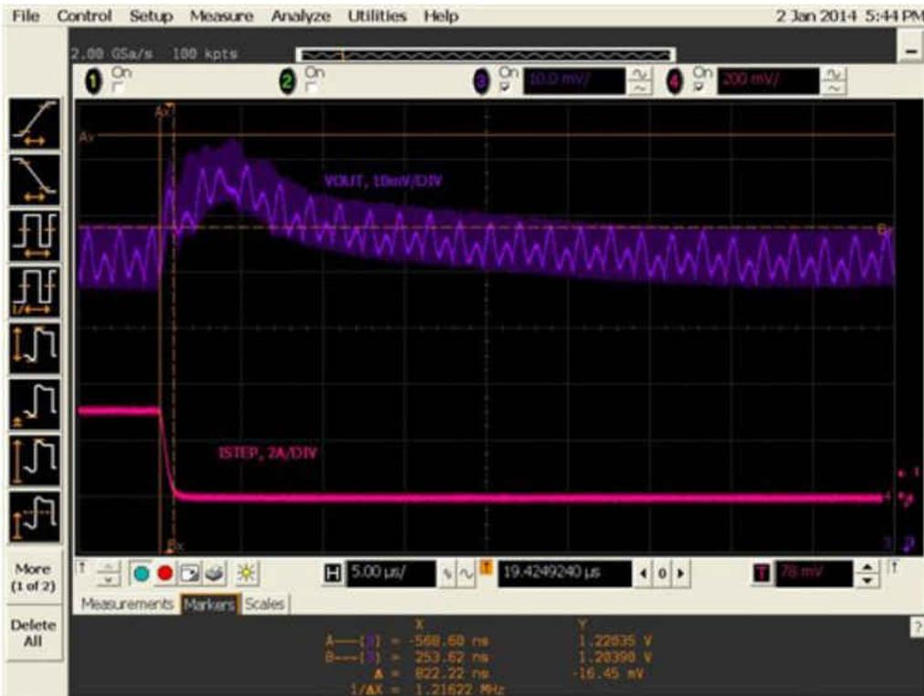
Figure 4-2. Step-Down Load Transient Response
