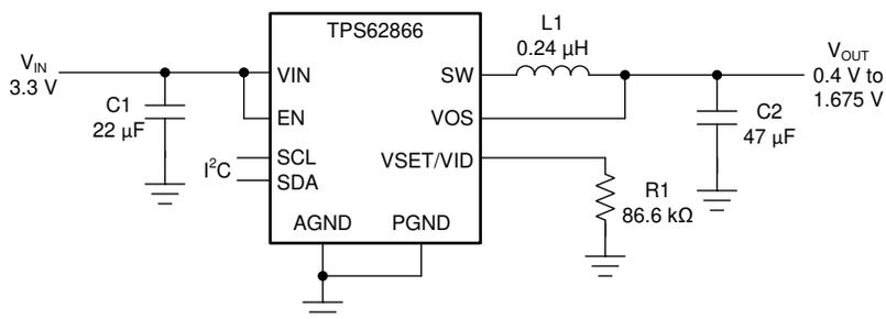
**Figure 2-1. TPS62866 Reduces Component Count Using the VSET Pin and I2C Communication**
