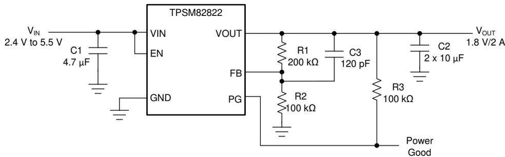
**Figure 3-3. TPSM82822 Power Module Integrates the Inductor to Provide a Small Solution Size**
