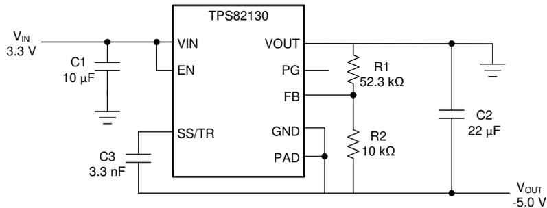
Figure 4-2. TPS82130 in an Inverting Buck-Boost Topology
