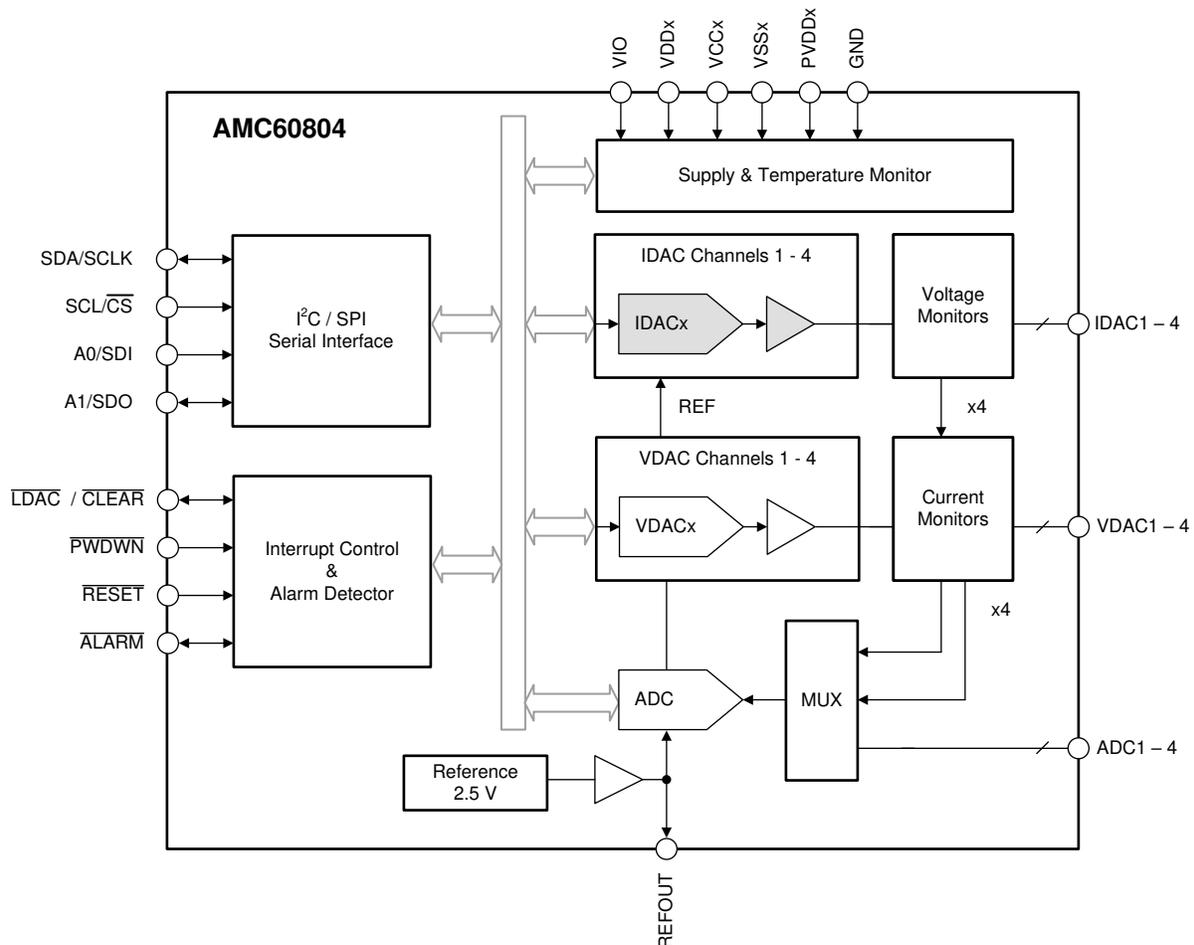
Figure 4-1. AMC60804 Provides Comprehensive Bias and Control for EML Structures
