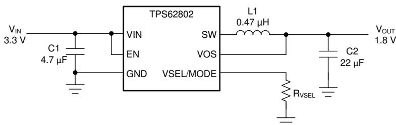
Figure 3-1. TPS62802 Reduces Component Count Using the VSEL Pin
