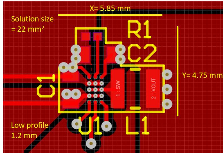
**Figure 2-2. 6-A TPS62866 Powers the DSP Core Rail With Its I<sup>2</sup>C Interface and Small Solution Size**
