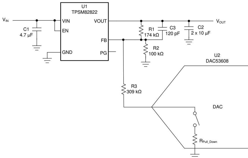
**Figure 6-1. DAC53608 Adjusts the TPSM82822 Output Voltage**
