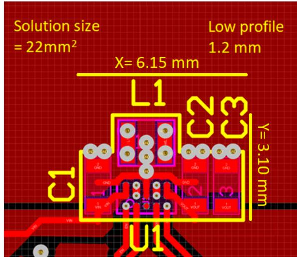
Figure 5-2. PCB Layout for the TPS63810 With a Solution Size of Only 22 mm<sup>2</sup>
