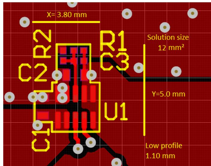
**Figure 3-4. TPSM82822 Power Module Integrates the Inductor to Provide a Small Solution Size**
