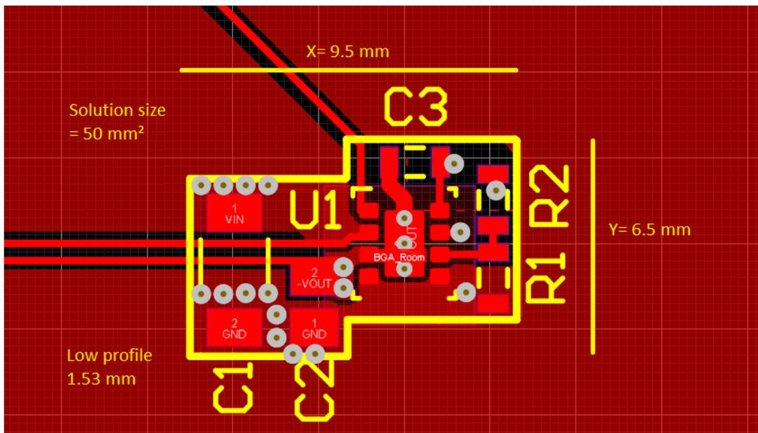
Figure 4-3. 3-A TPS82130 in an Inverting Buck-Boost Topology Powers the Negative Supply of an EAM With a Solution Size of Only 50 mm<sup>2</sup>
