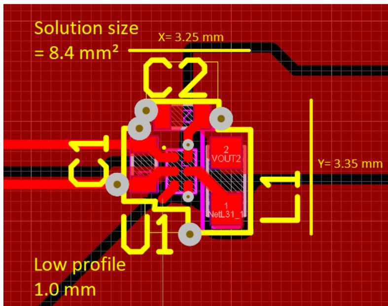
Figure 3-2. 1-A TPS62802 Powers Logic Circuitry Rails With a Tiny Solution Size
