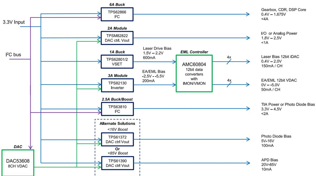
**Figure 1-1. Optical Module Power Tree With Control and Biasing Data Converters**
