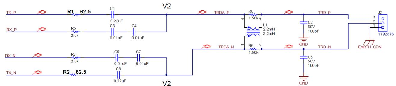
**Figure 4-2. 125 ohm Characteristic Impedance Cable Design**
