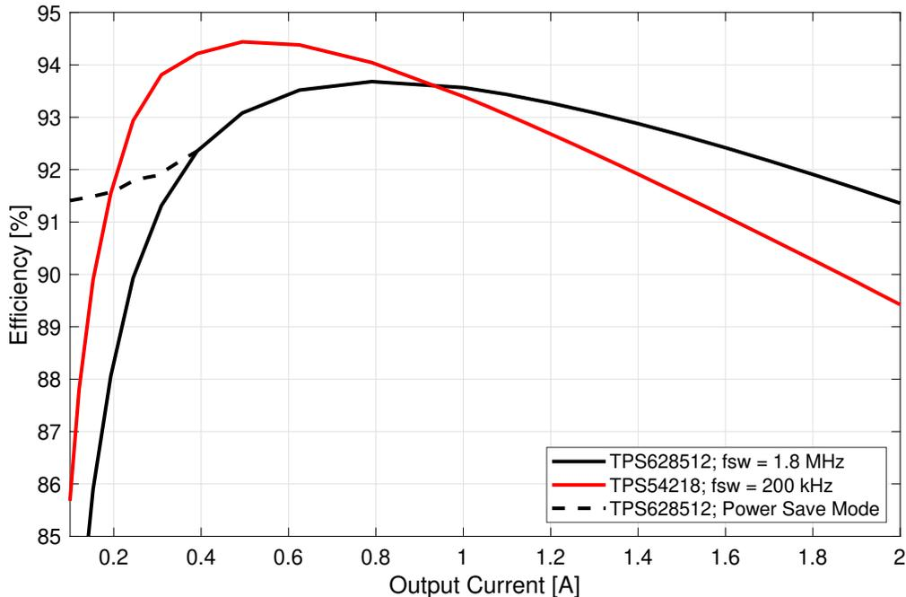
**Figure 3-1. Efficiency Comparison**
