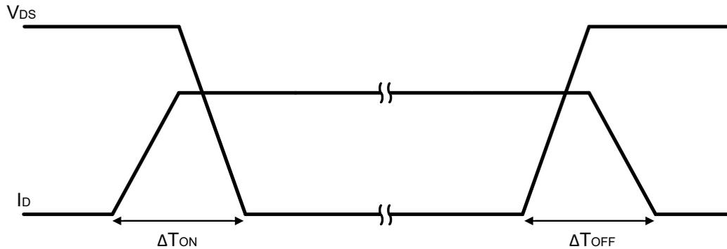
**Figure 2-1. MOSFET Turn-on and Turn-off**
