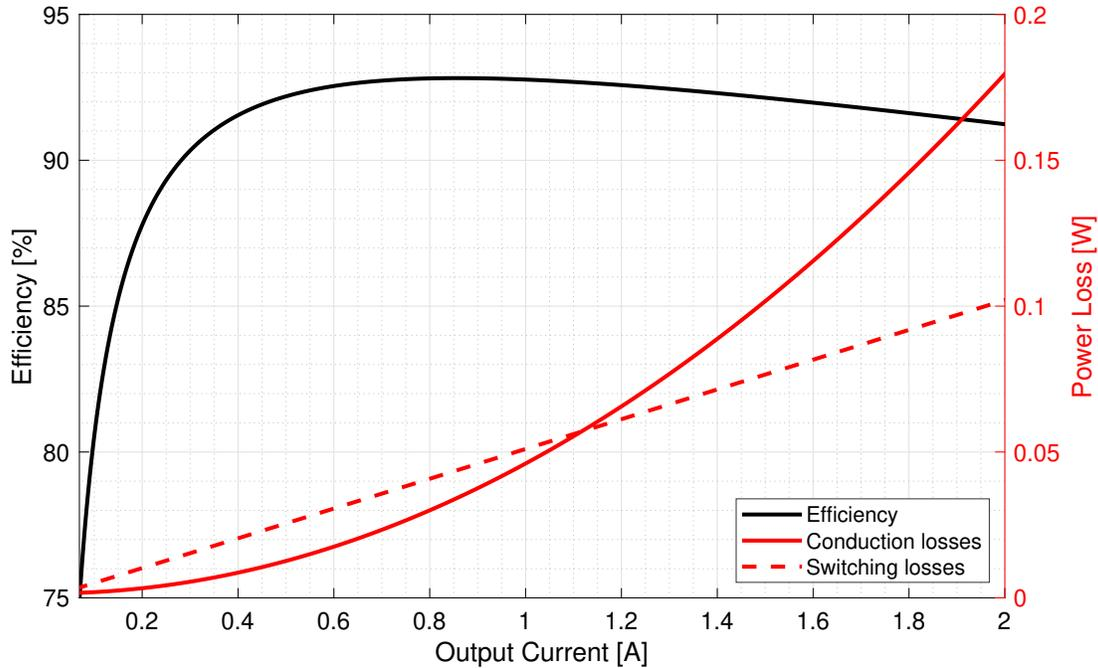
**Figure 2-2. How Conduction and Switching Losses Vary with Output Current**
