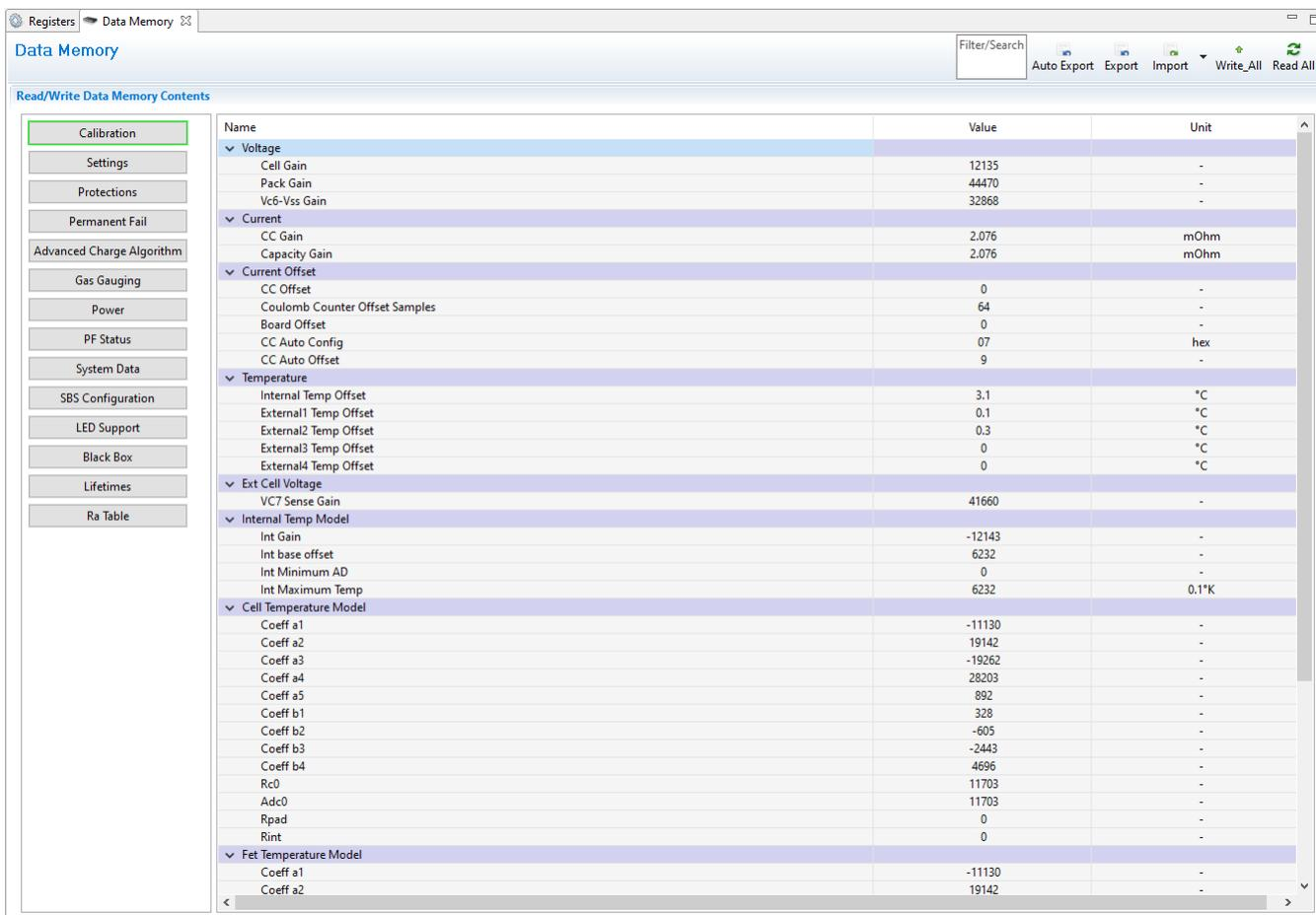
The screenshot shows the 'Data Memory' window in the TI software. The 'Calibration' tab is selected in the left-hand menu. The main area displays a table of parameters with columns for Name, Value, and Unit. The parameters are grouped into categories like Voltage, Current, Current Offset, Temperature, Ext Cell Voltage, Internal Temp Model, Cell Temperature Model, and Fet Temperature Model.
