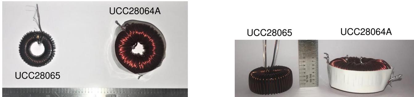
**Figure 11. Boost Inductor Comparison**
