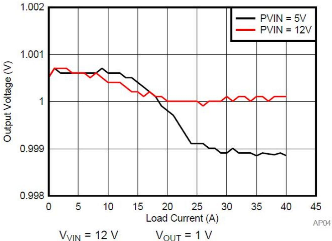
**Figure 1. TPS546D24A Load Regulation**
