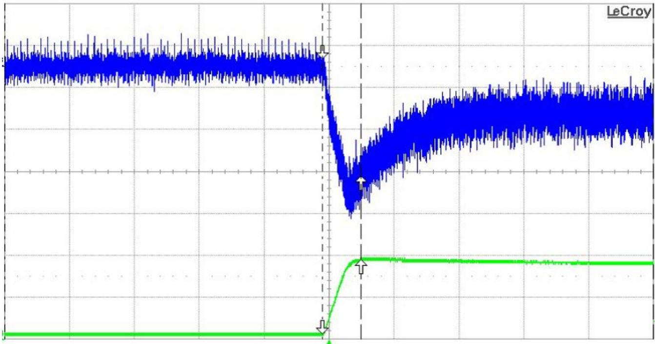
**Figure 3. Load Transient for Typical Converter without Internal Voltage Divider**
