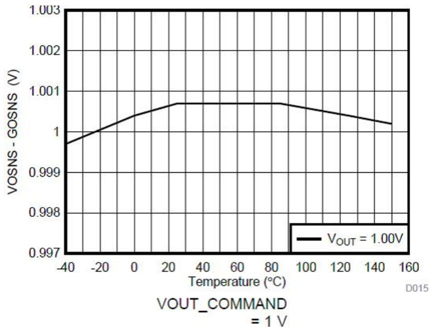
**Figure 2. Output Voltage Versus Junction Temperature**
