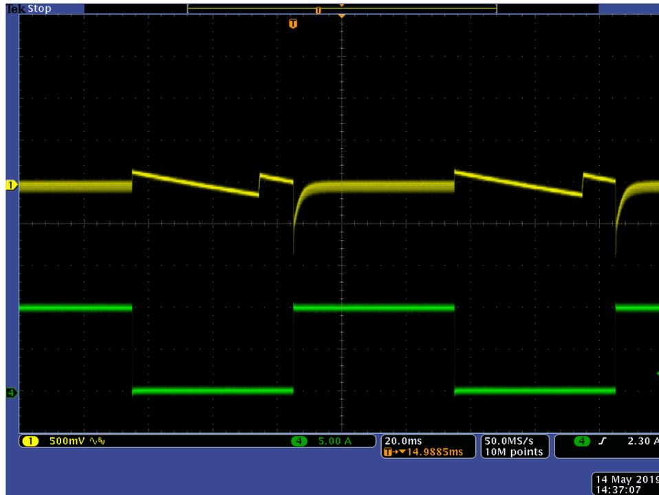
Figure 13. 10 mA to 10 A Transient (Ch1=V<sub>OUT</sub>; Ch4 = I<sub>OUT</sub>)
