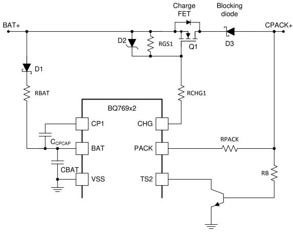
Figure 24. Wakeup Circuit with Blocking Schottky
