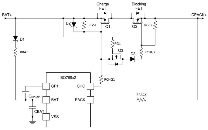
Figure 10. Charge Path Blocking FET
