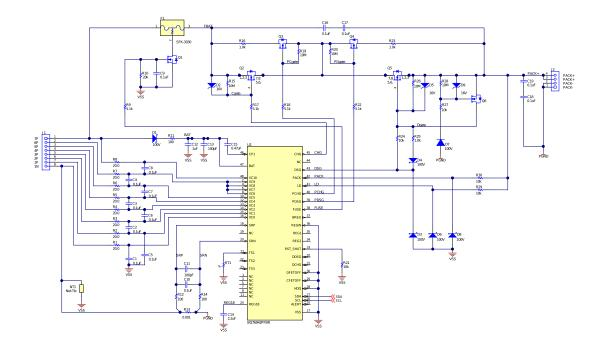
Figure 1. Typical 7S Series FET Schematic
