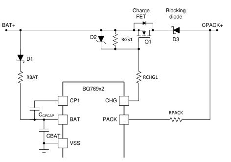
Figure 9. Blocking Discharge in Charge Path with Schottky
