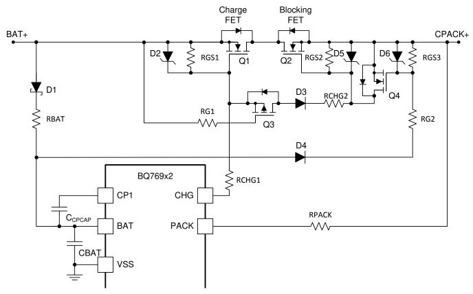
Figure 15. Charge Path with Blocking and Clamp FETs
