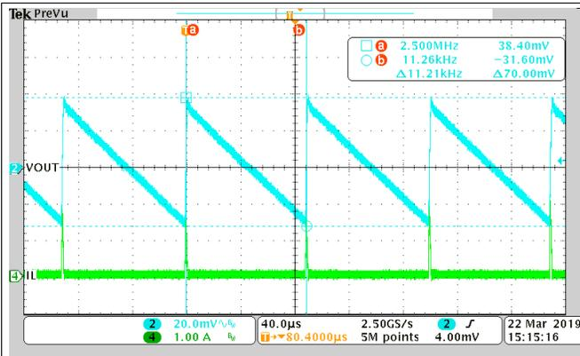
Figure 12. Eco-mode, 20 mA,  $F_{RIPPLE} = 11.2$  kHz, in Audio Frequency Range
