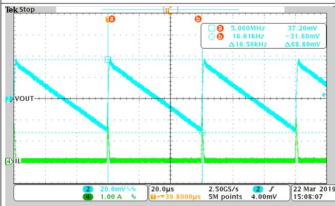
Figure 14. Eco-mode, 30 mA,  $F_{RIPPLE} = 16.6$  kHz, in Audio Frequency Range
