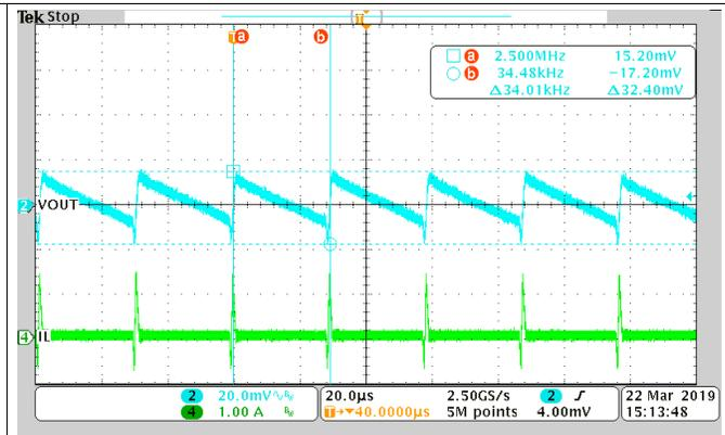
Figure 13. OOA Mode, 20 mA,  $F_{RIPPLE} = 34$  kHz, Out-of-Audio Frequency Range
