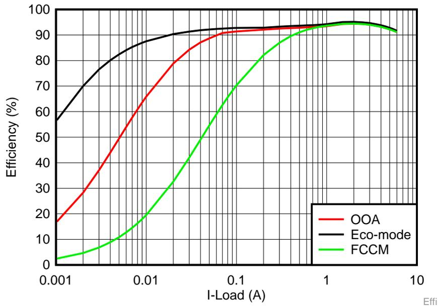
**Figure 19. Efficiency Comparison in Eco-mode, OOA, FCCM Mode**
