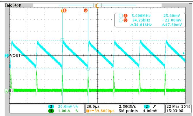
Figure 17. OOA Mode, 40 mA,  $F_{RIPPLE} = 34$  kHz, Out-of-Audio Frequency Range
