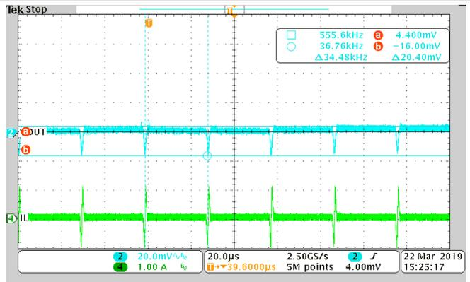
Figure 7. OOA Mode, 0 A,  $F_{\text{RIPPLE}} = 34.5$  kHz, Out-of-Audio Frequency Range
