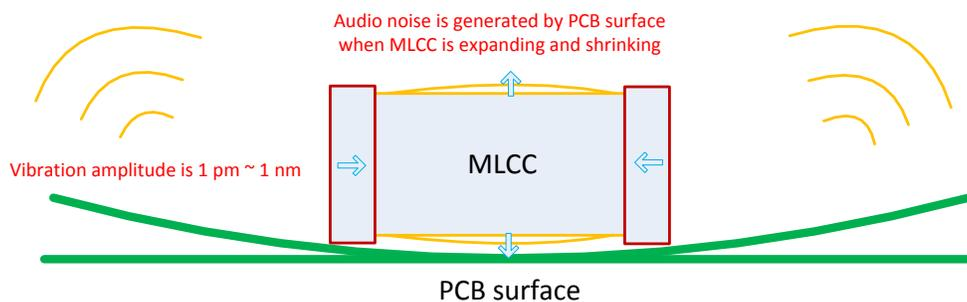
Figure 1. PCB Vibration by MLCC Electrostrictive Effect
