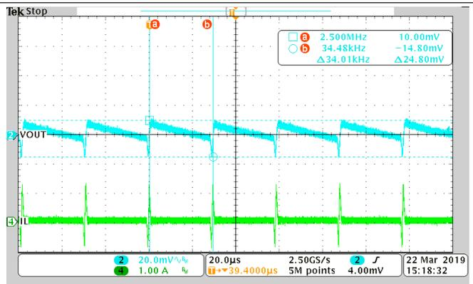
Figure 11. OOA Mode, 10 mA,  $F_{\text{RIPPLE}} = 34$  kHz, Out-of-Audio Frequency Range
