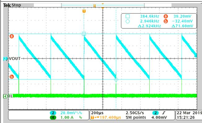
Figure 8. Eco-mode, 5 mA,  $F_{\text{RIPPLE}} = 2.9$  kHz, in Audio Frequency Range
