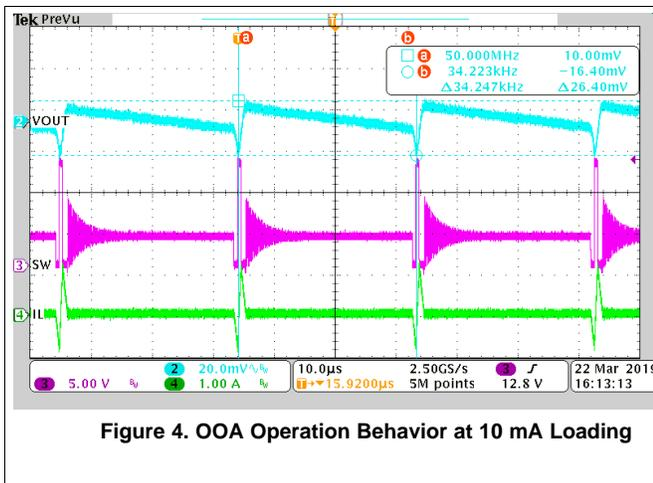
Figure 4. OOA Operation Behavior at 10 mA Loading
