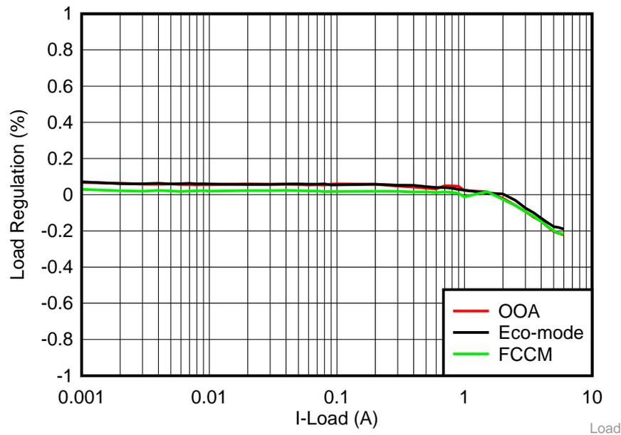
Figure 20. Load Regulation Comparison in Eco-mode, OOA, FCCM Mode
