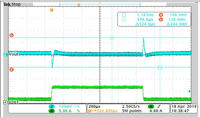
**Figure 24. 1 A to 6 A, OOA Mode,  $V_{pp} = 244$  mV**
