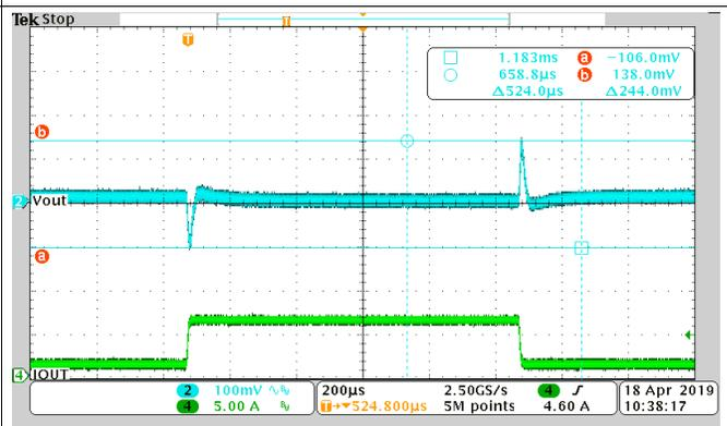
**Figure 26. 1 A to 6 A, FCCM Mode,  $V_{pp} = 244$  mV**
