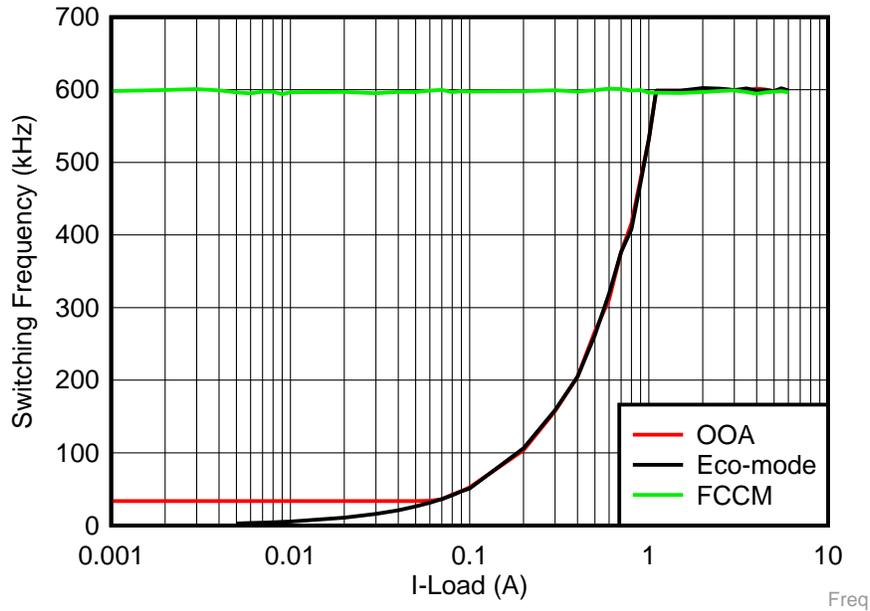
**Figure 18. Switching Frequency Comparison in Eco-mode, OOA, FCCM Mode**
