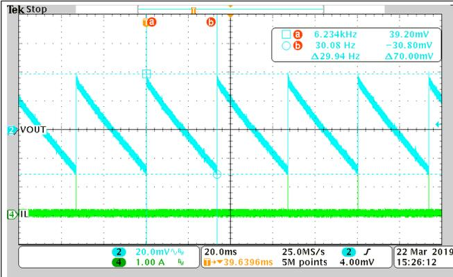
Figure 6. Eco-mode, 0 A,  $F_{\text{RIPPLE}} = 29.9$  Hz, in Audio Frequency Range
