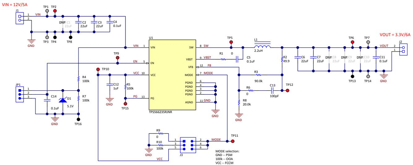
Figure 3. TPS566235EVM-036 Evaluation Module Schematic
