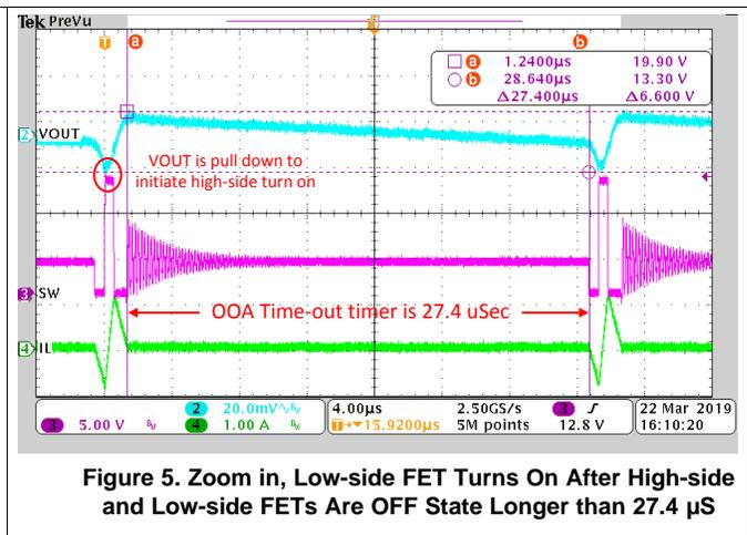
Figure 5. Zoom in, Low-side FET Turns On After High-side and Low-side FETs Are OFF State Longer than 27.4  $\mu$ S
