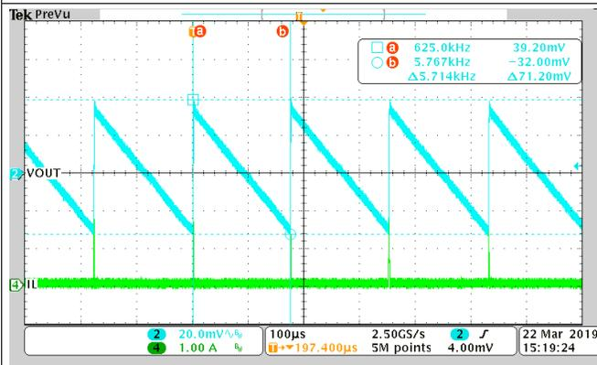
Figure 10. Eco-mode, 10 mA,  $F_{\text{RIPPLE}} = 5.7$  kHz, in Audio Frequency Range
