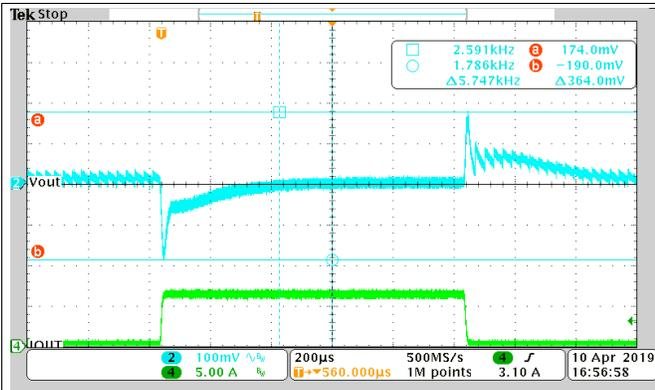
**Figure 23. 0 A to 6 A, OOA Mode,  $V_{pp} = 364$  mV**
