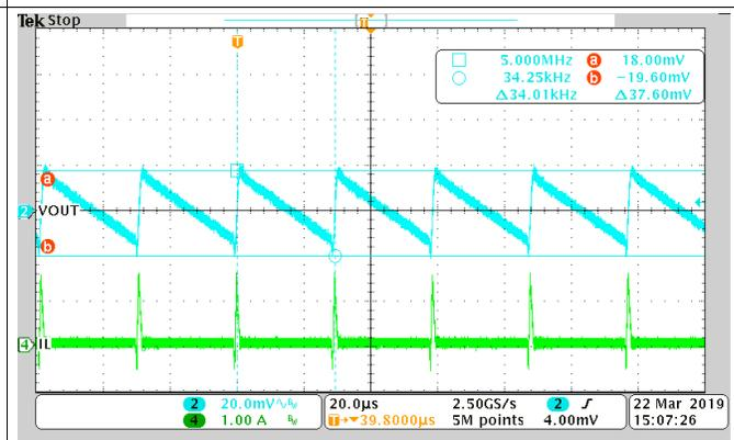
Figure 15. OOA Mode, 30 mA,  $F_{RIPPLE} = 34$  kHz, Out-of-Audio Frequency Range
