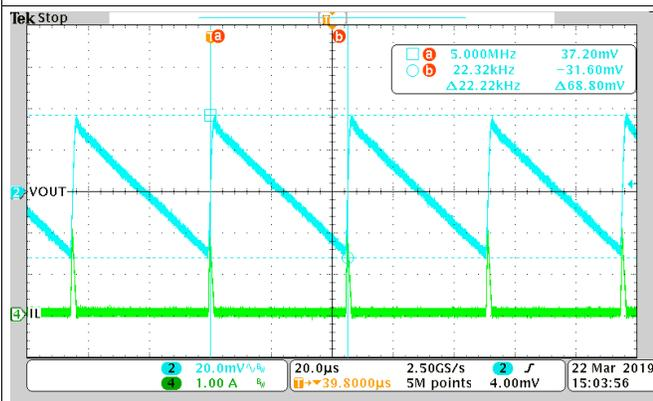
Figure 16. Eco-mode, 40 mA,  $F_{RIPPLE} = 22.2$  kHz, Out-of-Audio Frequency Range
