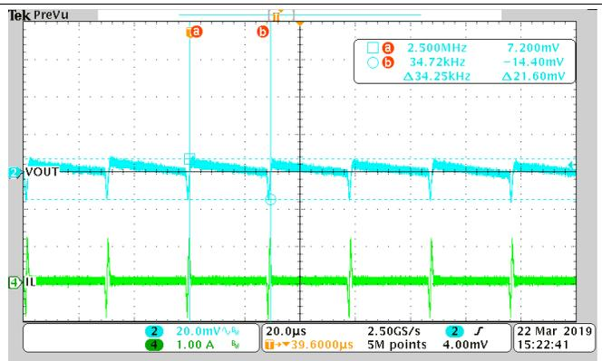
Figure 9. OOA Mode, 5 mA,  $F_{\text{RIPPLE}} = 34.3$  kHz, Out-of-Audio Frequency Range
