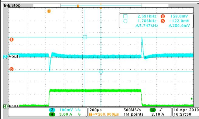
**Figure 25. 0 A to 6 A, FCCM Mode,  $V_{pp} = 280$  mV**
