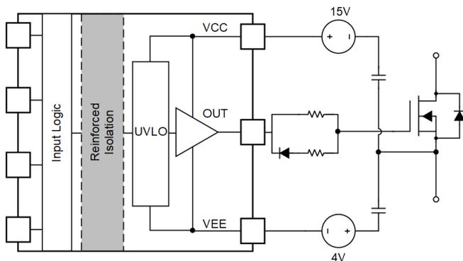
**Figure 2. Isolated driver with UVLO referenced to VEE.**
