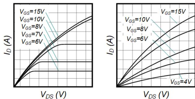
Figure 1. I-V Curves for a Si MOSFET (left) and SiC MOSFET (right).
