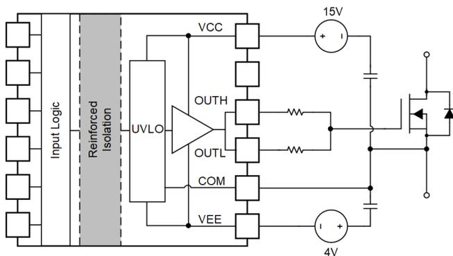
**Figure 3. Isolated driver with UVLO referenced to COM**
