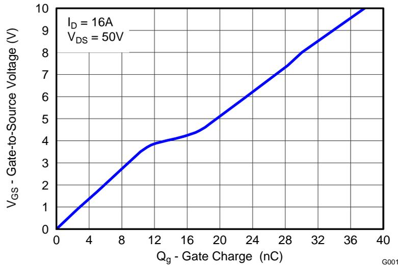
Figure 1. CSD19531 Gate Charge vs V<sub>GS</sub>
