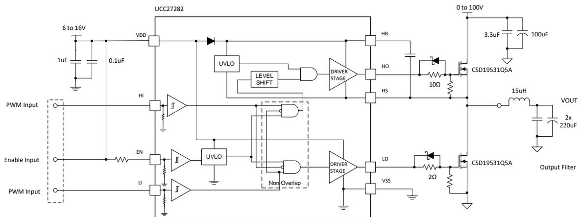
Figure 3. UCC27282 Sync-Buck Test Circuit
