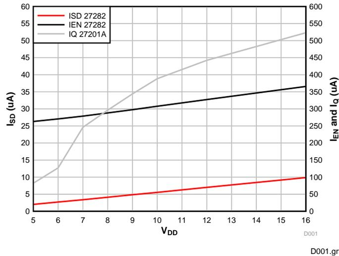
Figure 8. UCC27282 I<sub>EN</sub>, I<sub>SD</sub>, and UCC27201A I<sub>Q</sub>
