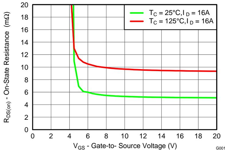
Figure 2. CSD19531 R<sub>DS(on)</sub> vs V<sub>GS</sub>
