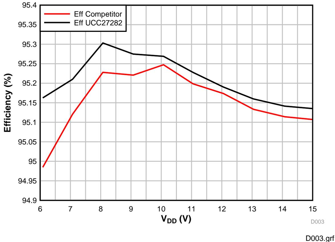
Figure 7. UCC27282 and Competitor Sync-Buck Efficiency vs  $V_{DD}$
