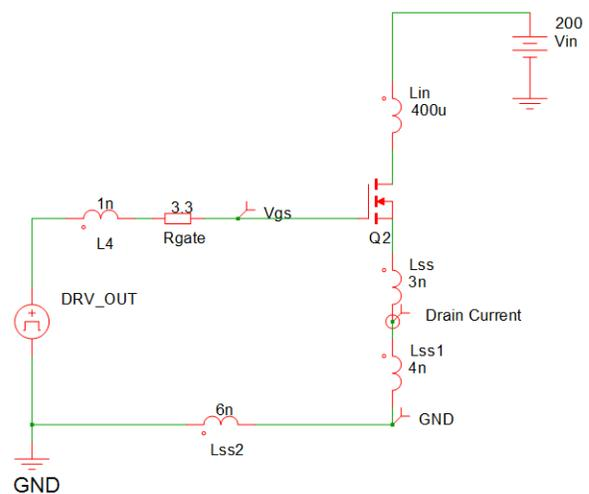
Figure 2. Example Simulation of a Simplified Low-side Gate Drive Power Stage
