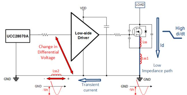
Figure 1. Simplified Schematic of a Low-side Gate Drive Using UCC27511A
