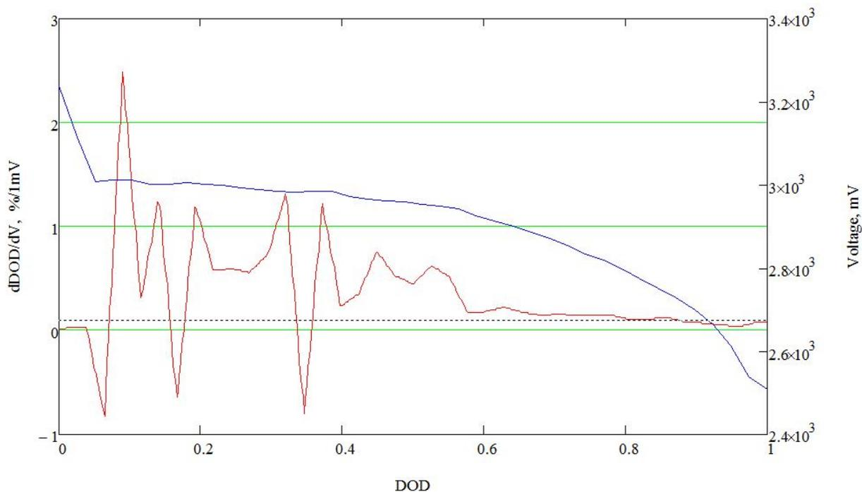
Figure 4. DOD vs OCV Error of the  $\text{LiMnO}_4$  Cell with bq35100
