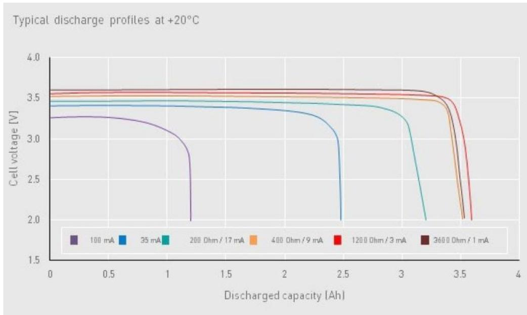
**Figure 2. Discharge Profiles of a Lithium Thionyl Chloride Cell (Source: SAFT)**
