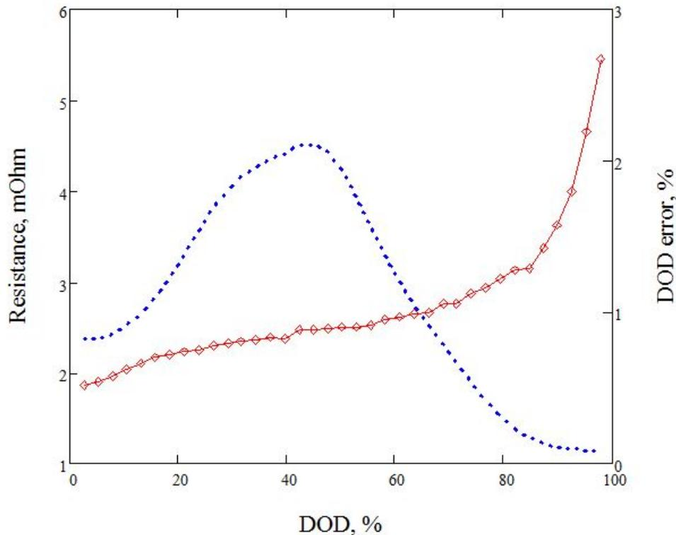
**Figure 5. Resistance and DOD Error vs DOD Percentage**
