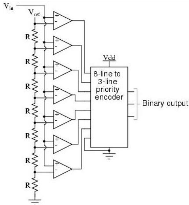
**Figure 3. Flash ADC Architecture**
