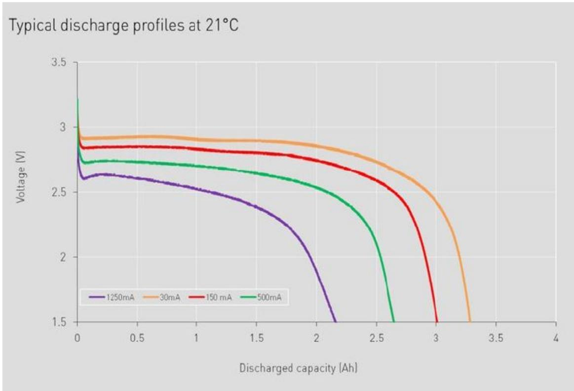
Figure 1. Discharge Profiles of a Lithium Manganese Dioxide Cell (Source: SAFT)
