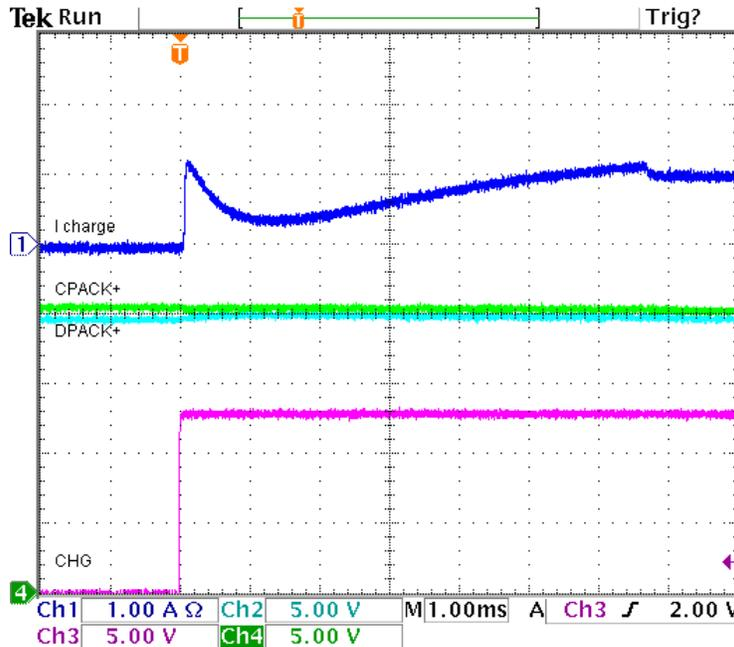
Figure 18. JFET Circuit Turn On
