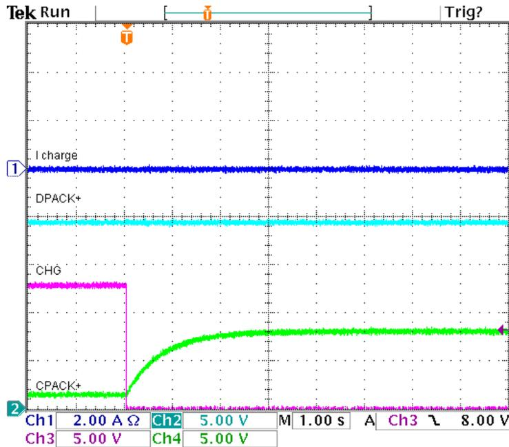
Figure 10. Diode Leakage Example in Hibernate Mode
