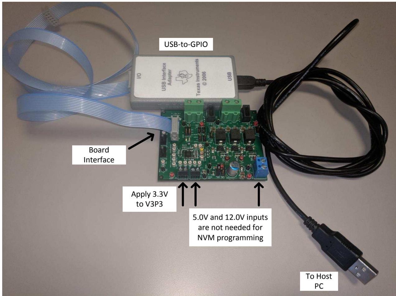
Figure 1. Hardware Connections
