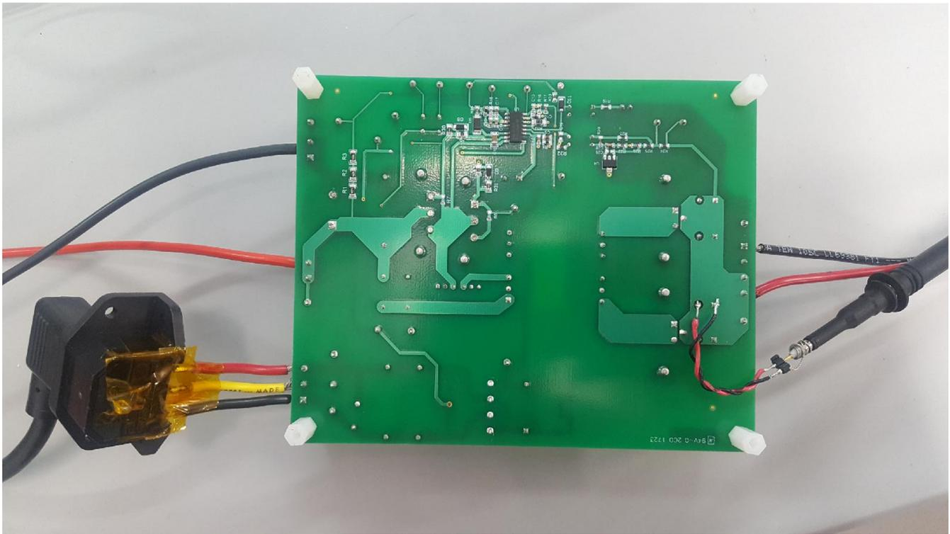
Figure 5. Tip and Barrel Probing
