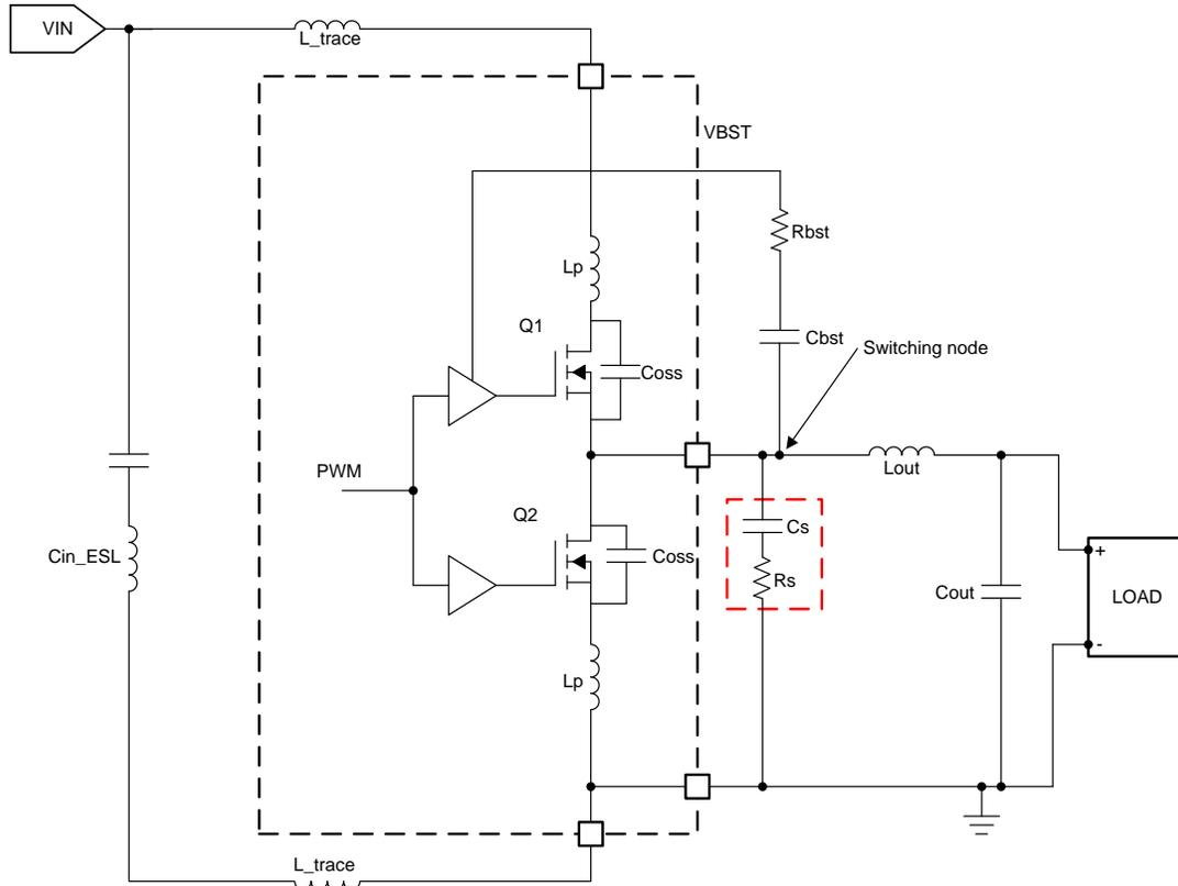
Figure 4. RC Snubber Added Circuit With Parasitic Components
