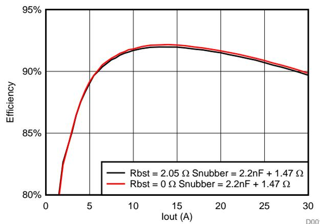
Figure 12. Boot Resistor Effects on Efficiency
