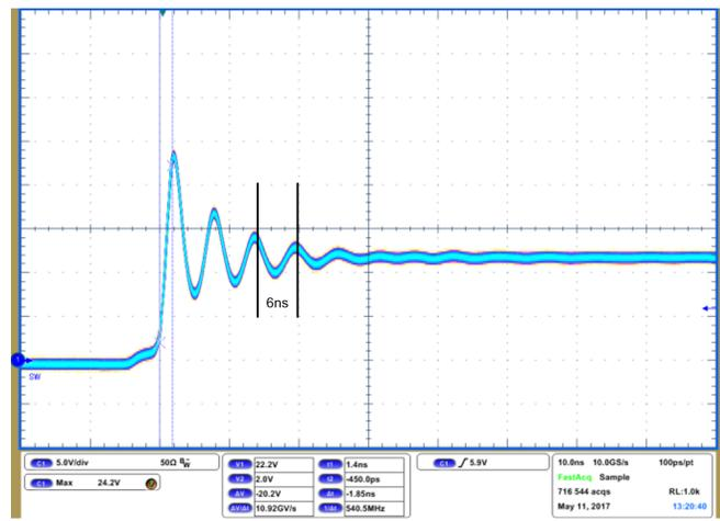
Figure 11.  $R_{bst} 0\ \Omega + 0.1\ \mu\text{F}$  and  $1.47\ \Omega + 2.2\ \text{nF}$  Snubber
