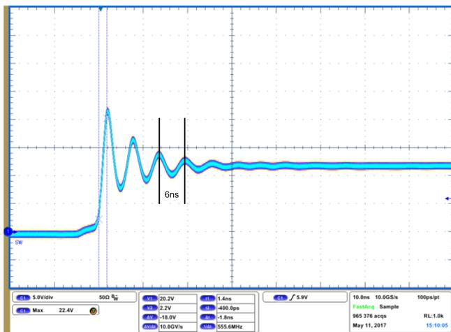
Figure 10.  $R_{bst} 2.05\ \Omega + 0.1\ \mu\text{F}$  and  $1.47\ \Omega + 2.2\ \text{nF}$  Snubber
