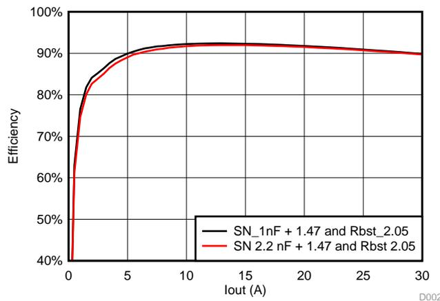
Figure 13. Efficiency Comparison When Snubber Capacitance  $C_s$  Changes
