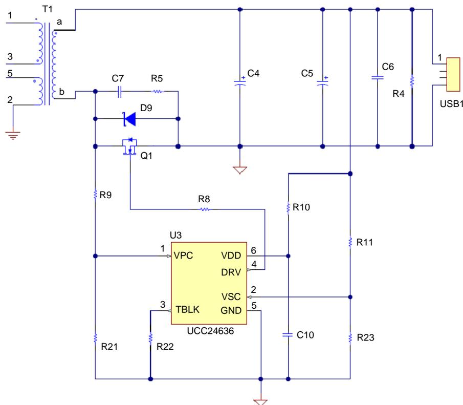
**Figure 5. PMP11600 Part of Circuit Showing SR With a Schottky in Parallel**
