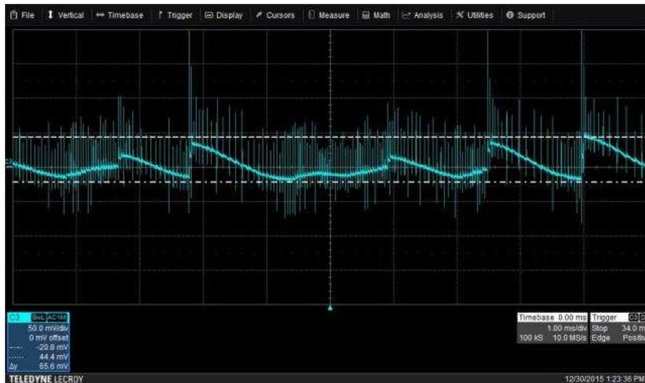
Figure 3. Output Voltage Ripple Irregular Waveforms
