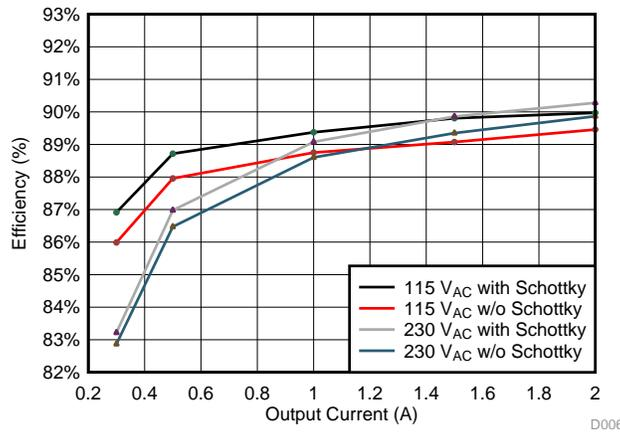
Figure 6. PMP11600 5V2A Converter Efficiency Test Result
