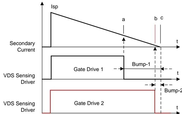
**Figure 4. Bump Time Setup With the UCC24636**
