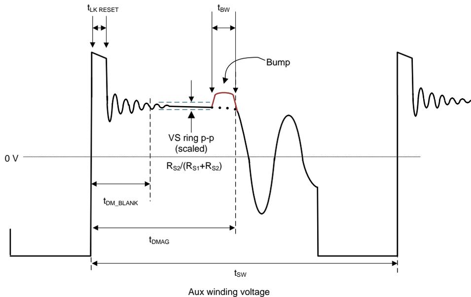
Figure 2. De-mag Time Partition and Body Diode Conduction Bump
