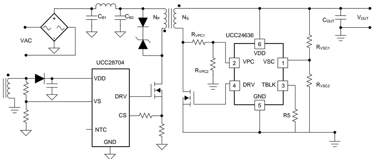
Figure 1. Functional Circuit Diagram
