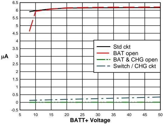
Figure 4. Shutdown Current Comparison
