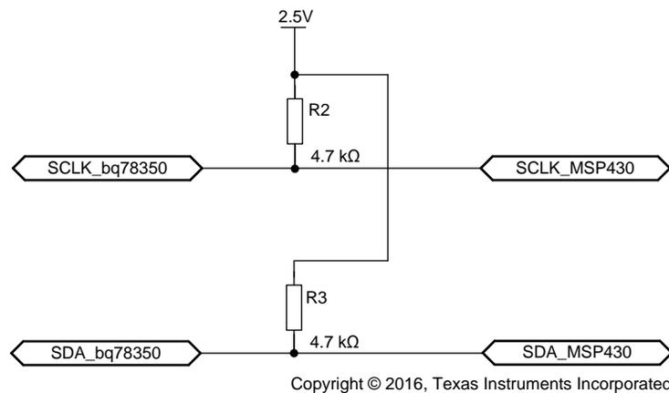
**Figure 2. Level-Shifter Schematic (MSP430G2553 and bq78350)**
