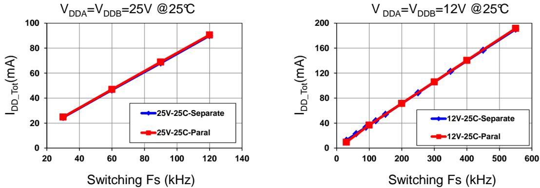
Figure 11. VDD Total Operating Current vs. F<sub>s</sub> at 25°C
