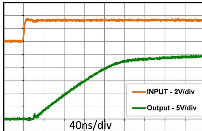
**Figure 1. Single Channel Driving 30-nF Load Capacitance**
