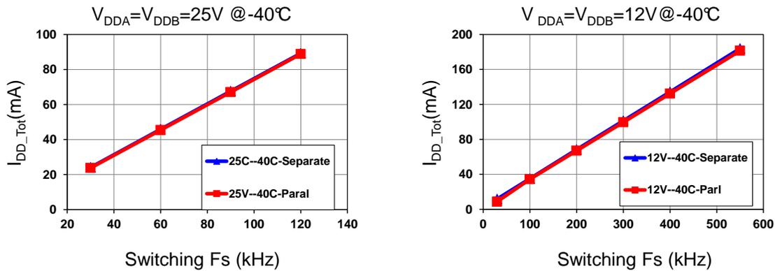
Figure 12. VDD Total Operating Current vs. F<sub>s</sub> at -40°C
