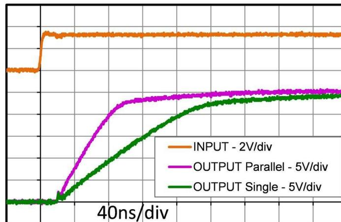
Figure 15. UCC21520 Single Channel Driving 30-nF Load Capacitance
