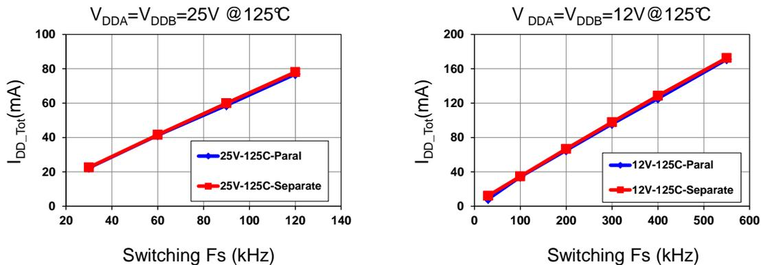
Figure 13. VDD Total Operating Current vs. F<sub>s</sub> at 125°C
