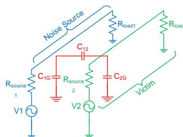
Figure 3. Capacitive Coupling in Electric Circuit
