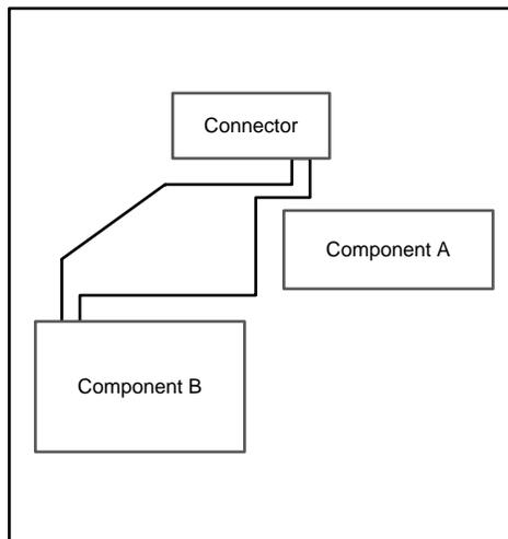
**Figure 9. Unmatched Differential Pair Routing**
