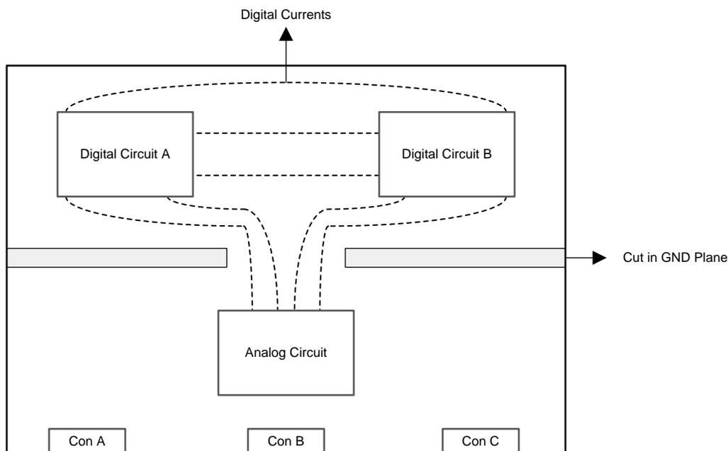
**Figure 10. Isolated Analog Section Using Cut in Ground Plane to Improve Performance**
