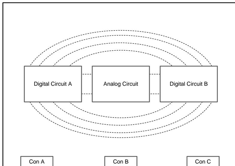
**Figure 11. High Frequency Digital Noise Induced in Analog Circuit**
