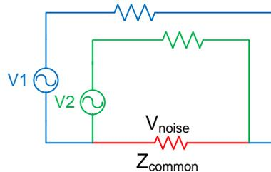
**Figure 4. : Circuit Showing Common Impedance Between Noise Source and Victim**
