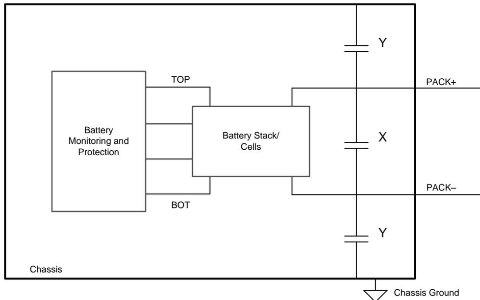
**Figure 5. Battery Pack with X and Y Capacitors**
