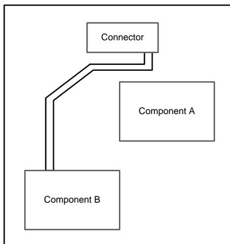
**Figure 8. Matched Differential Pair Routing**
