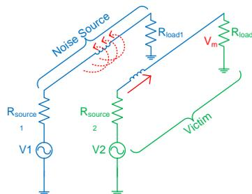
Figure 2. Inductive Coupling in Electric Circuit
