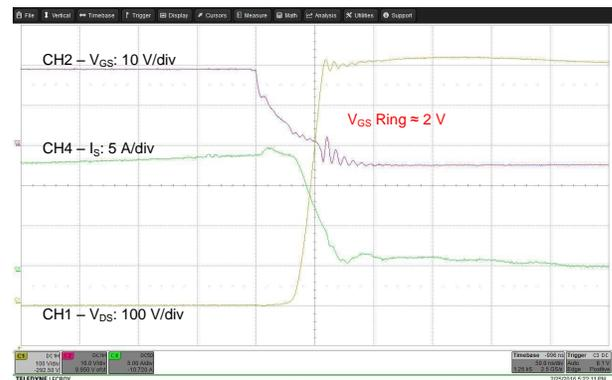
Figure 10.  $V_{DS}$ ,  $V_{GS}$ ,  $I_S$ , Reduce Driver Sink Current
