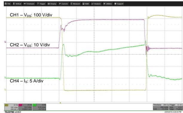
Figure 6.  $V_{DS}$ ,  $V_{GS}$ ,  $I_S$  Switching Cycle
