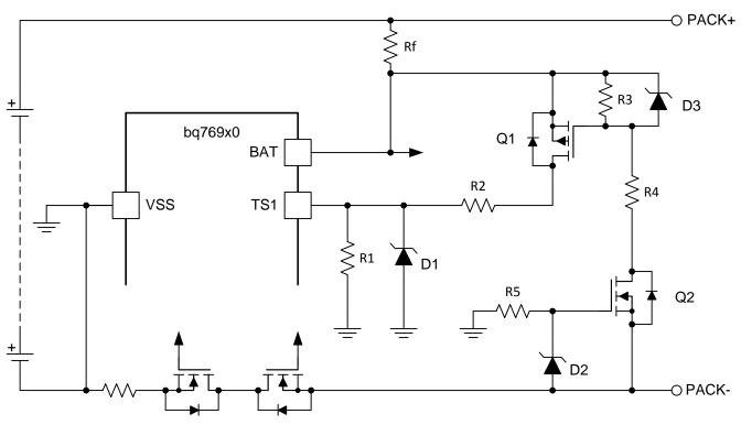
Figure 4. Pack Terminal Boot Circuit
