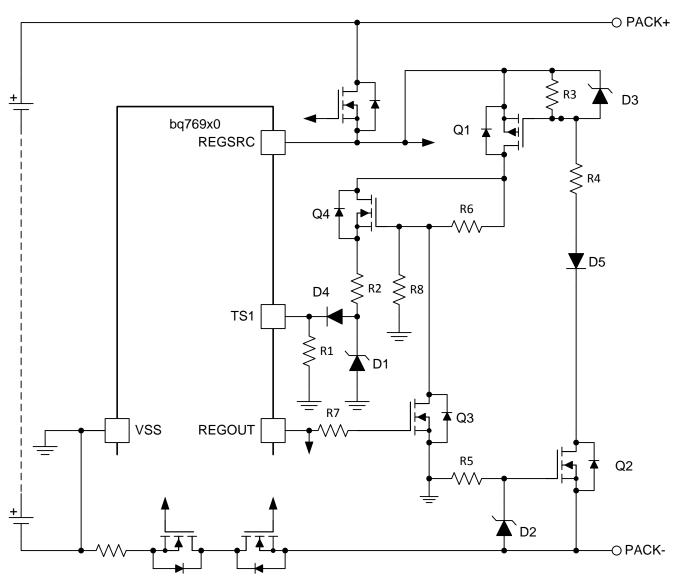
Figure 5. Pack Boot Switch From REGSRC
