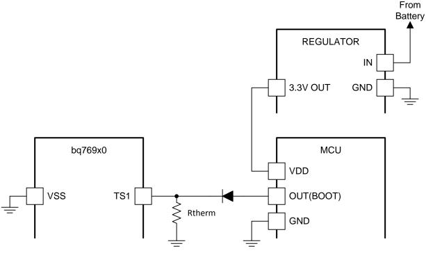
Figure 1. Independently Powered MCU Boot
