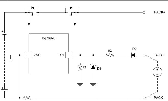
Figure 3. External Boot Signal, High-Side Switch
