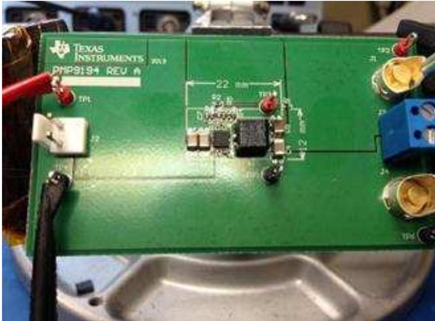
**Figure 9. TPS54020 PMP9194 with HotRod Package in Place**
