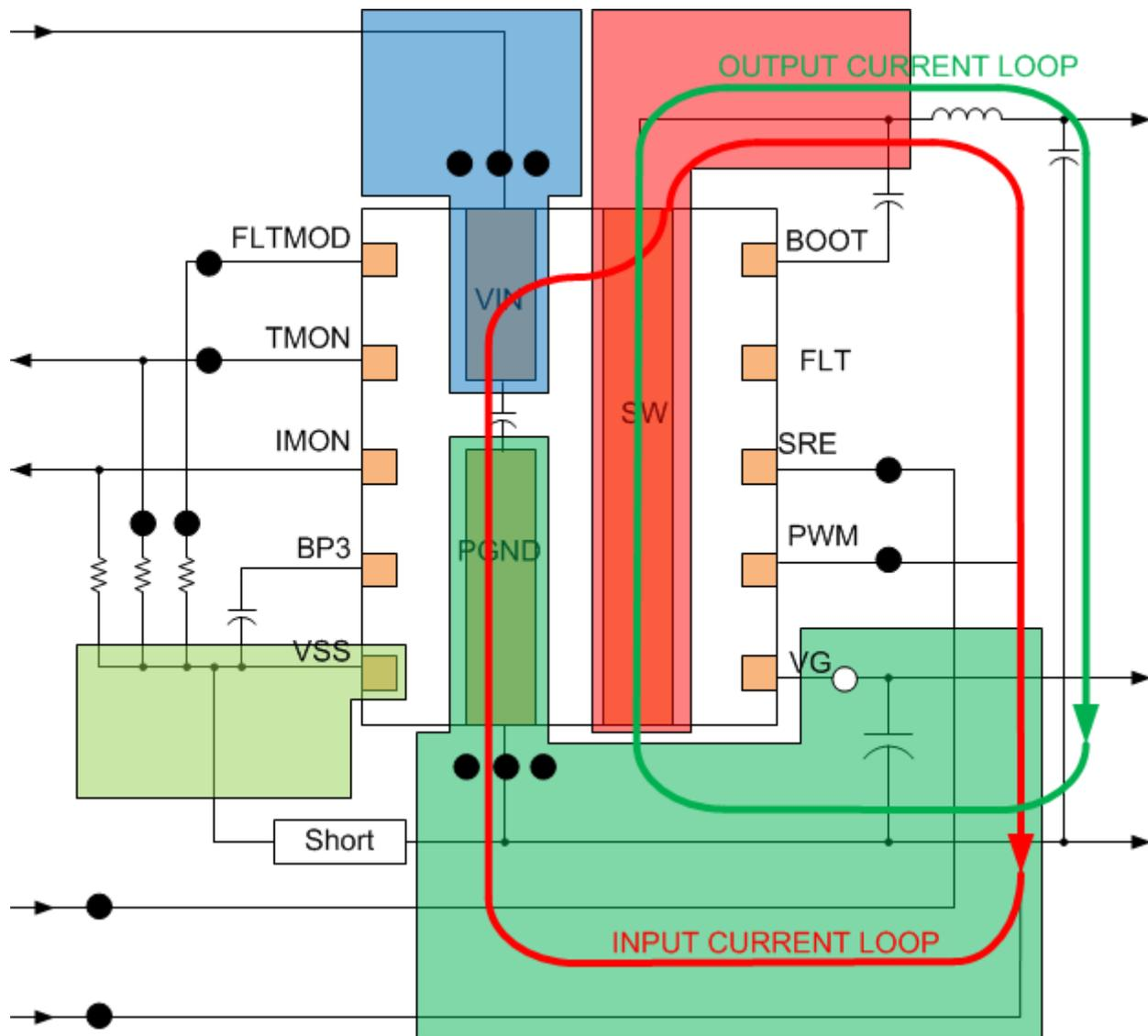
**Figure 6. Application Layout Example**
