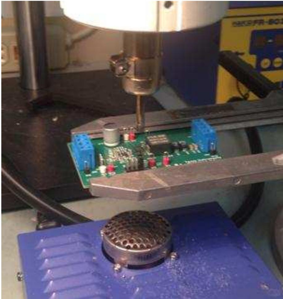
**Figure 10. Manual Rework Station for HotRod/QFN Package Devices**
