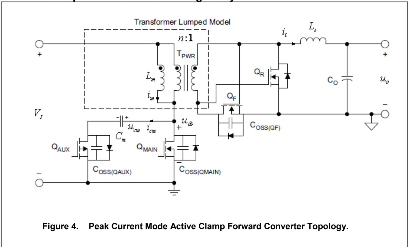
Figure 4. Peak Current Mode Active Clamp Forward Converter Topology.
