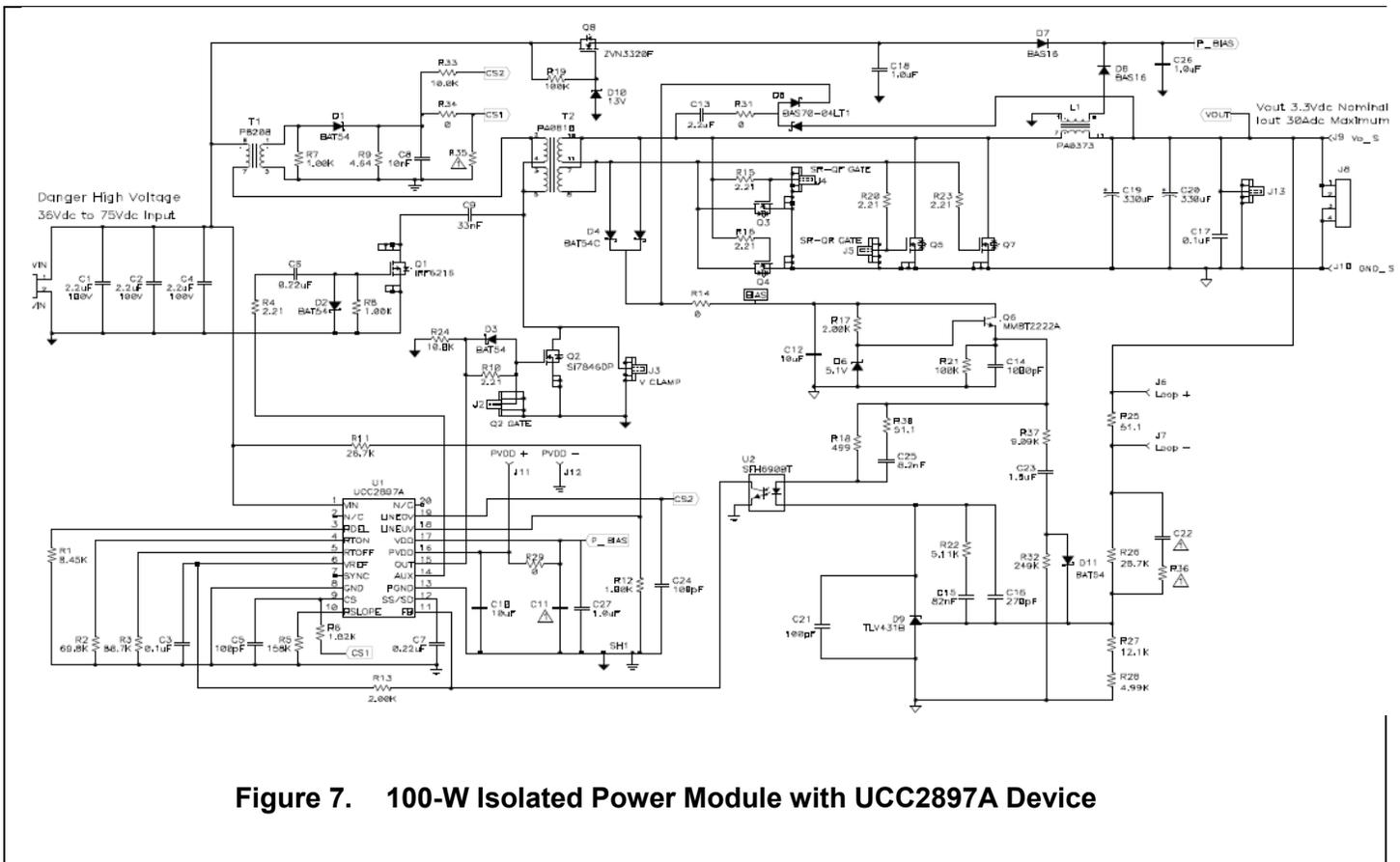
T1: Current transformer specification is: turn ratio is 1:100;
