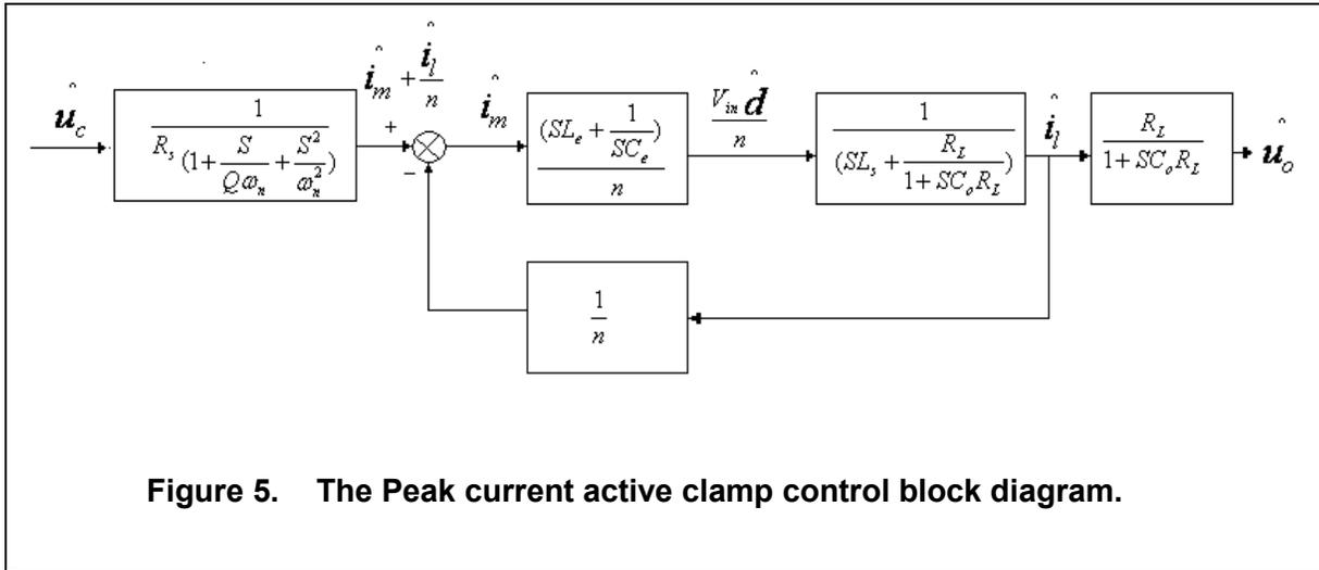
**Figure 5. The Peak current active clamp control block diagram.**
