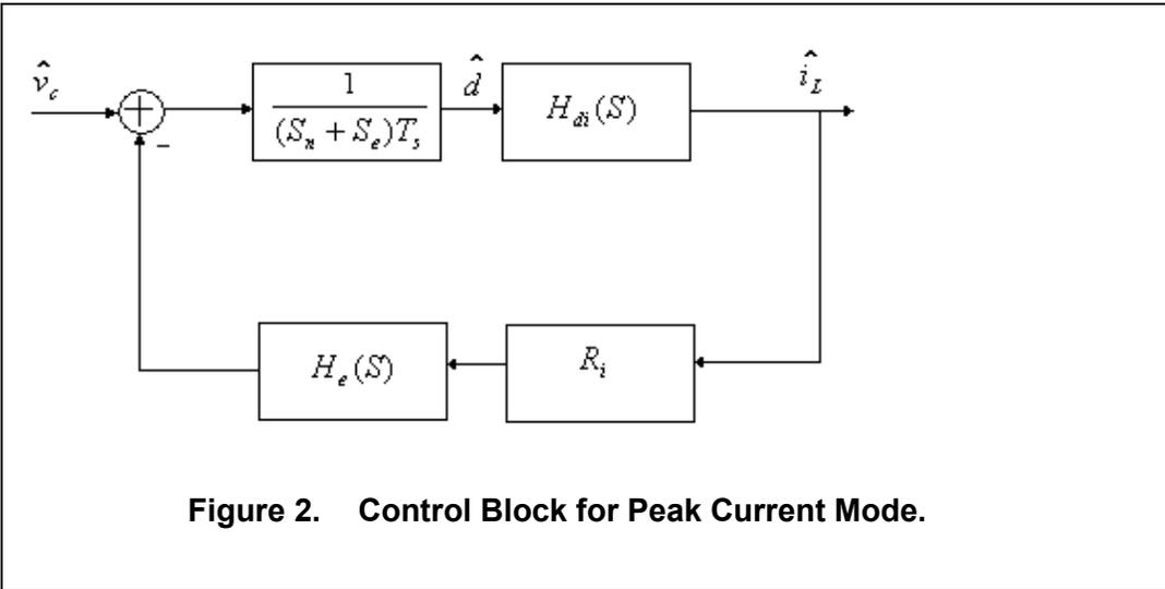
Figure 2. Control Block for Peak Current Mode.
