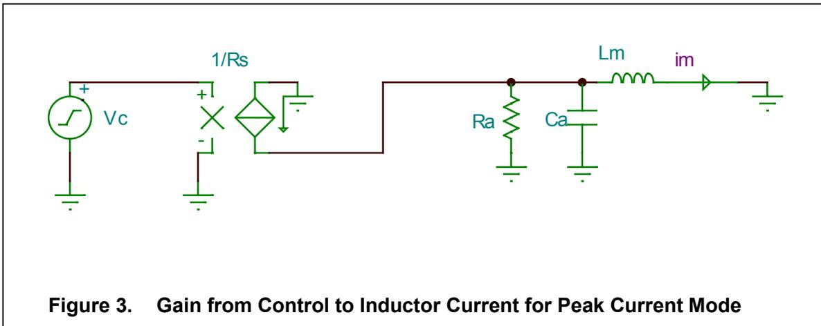
Figure 3. Gain from Control to Inductor Current for Peak Current Mode
