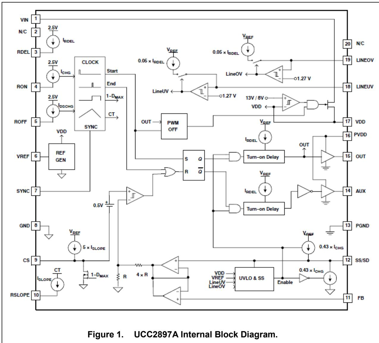
Figure 1. UCC2897A Internal Block Diagram.
