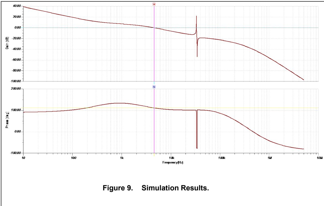
Figure.9 showed the cross-over frequency is 4.5 kHz, and phase margin is 111 degrees.
