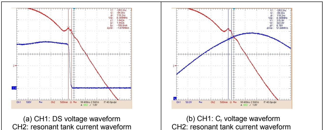
**Figure 6. Resonant Tank Current, DS Voltage and  $V_{Cr}$  Waveform During ZVS**
