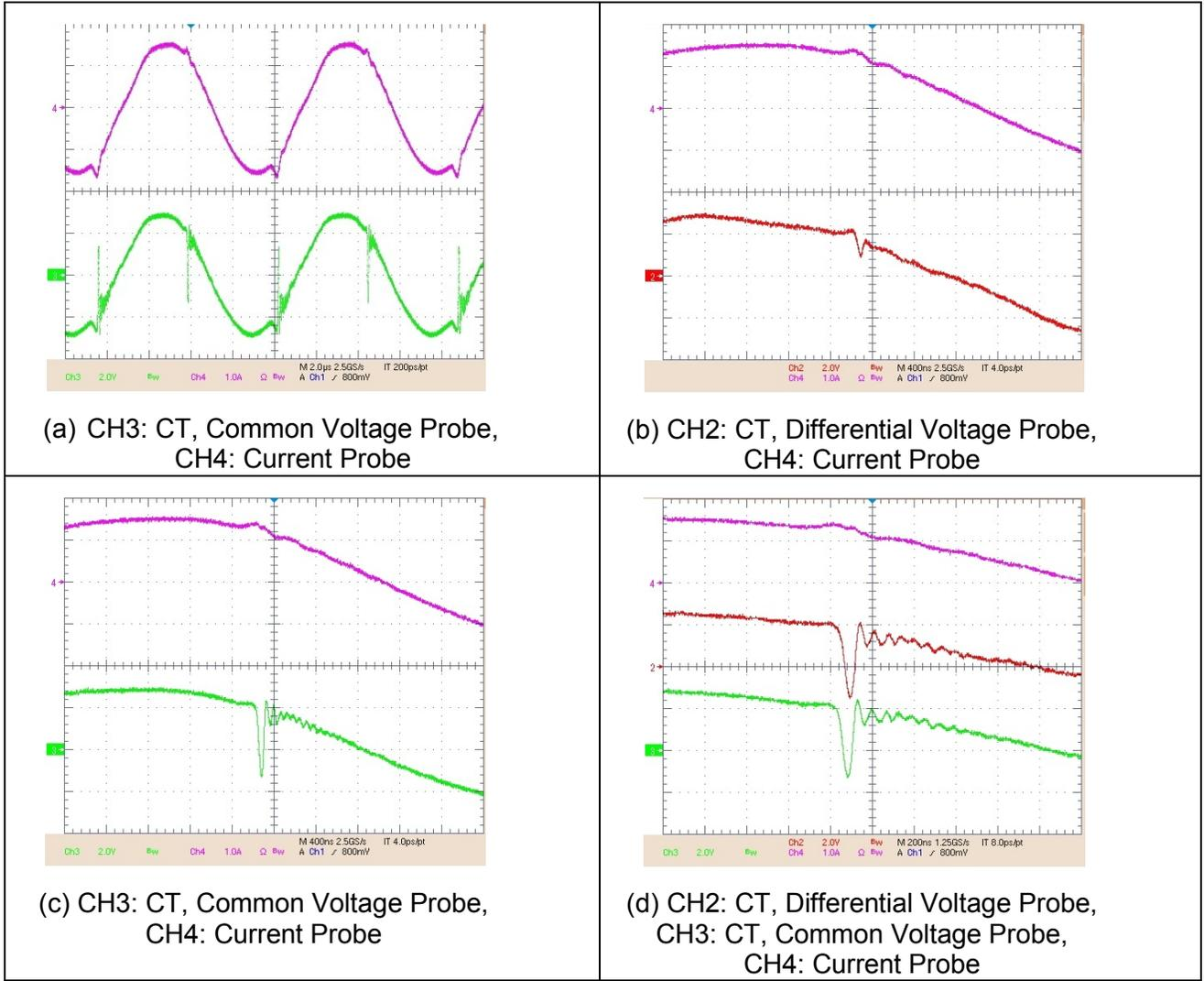
**Figure 5. Resonant Tank Current Measured by Different Methods**
