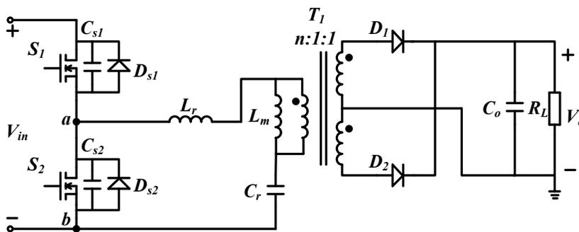
**Figure 1. LLC Resonant Half-bridge Converter**
