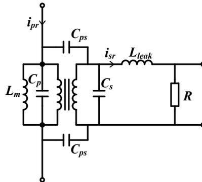
**Figure 4. Equivalent Model of Current Transformer**
