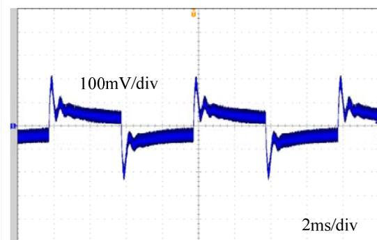
**Figure 13. Output Load Transient at 300-V Input**
