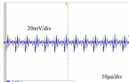
**Figure 11. Output Ripple at 300-V Input, Half Load**
