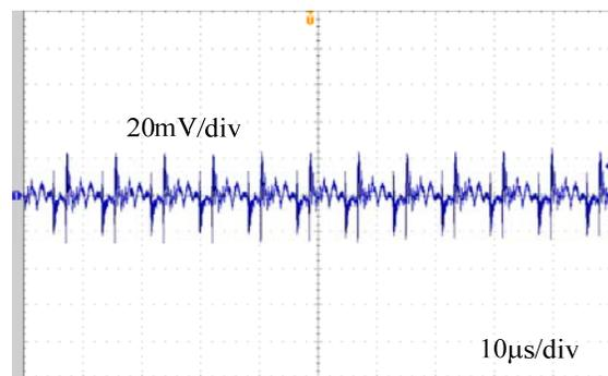
**Figure 10. Output Ripple at 300-V Input, Full Load**
