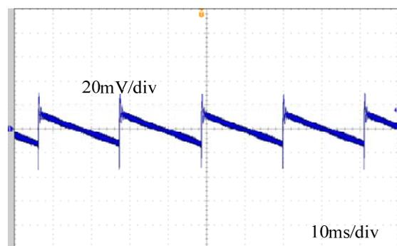
**Figure 12. Output Ripple at 300-V Input, No Load**
