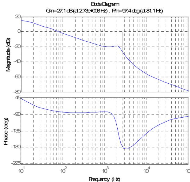
**Figure 5. Bode Figure of Original Loop Transfer Function**
