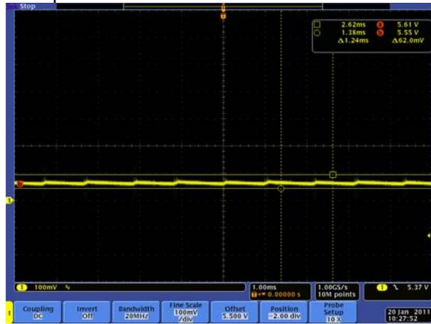
No Load ripple CH1:100mV/div at 230V input
