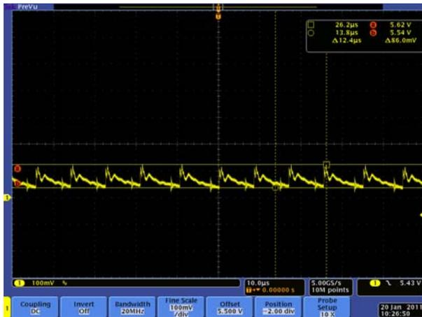
Full load ripple at 115V input CH1:100mV/div
