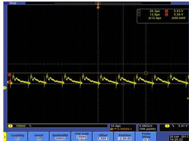
Full load ripple at 230V input CH1:100mV/div
