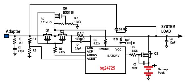
Figure 5. N-FETs Reverse Input Protection
