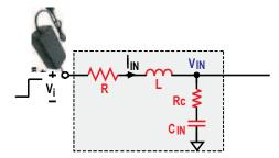
Figure 1. Simplified Equivalent Circuit During Adapter Insertion
