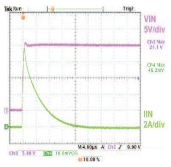
Figure 3. Adapter dc Side Hot Plug-in Test Waveforms
