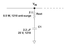
Figure 2. Recommended Input Filter Design
