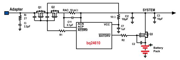
Figure 4. P-FETs Reverse Input Protection
