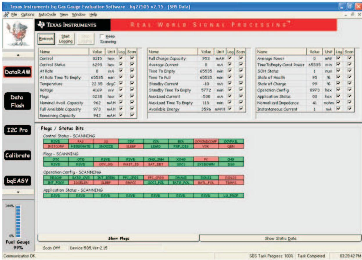
Figure 19. Sealed Mode for the bqEVSW DataRAM Window
