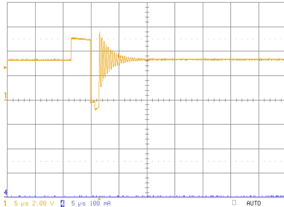
Fig 26: Switch node 5 Vin, 3.3V with no load
