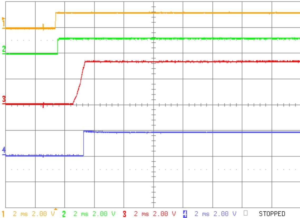
Fig 2: Start Up waveform with outputs fully loaded
