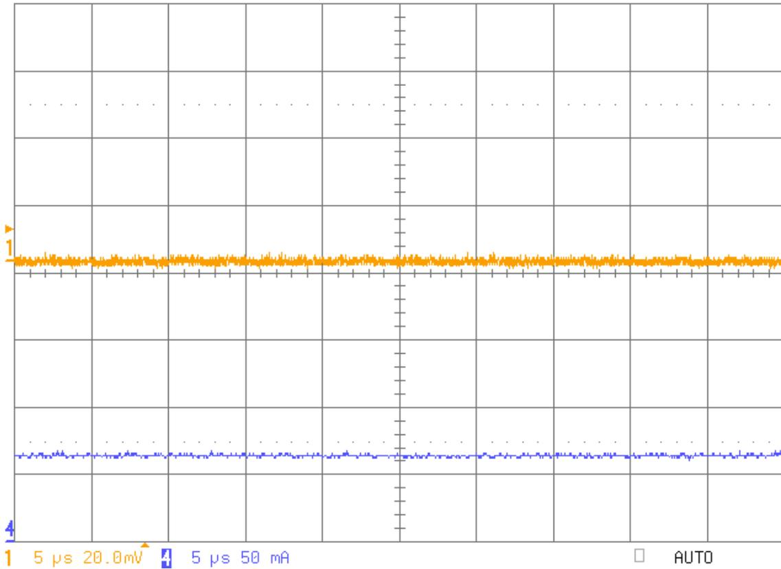
Fig 3: Output Ripple 1.2V @ 0.06A TPS 71701 LDO, 5V<sub>in</sub>
