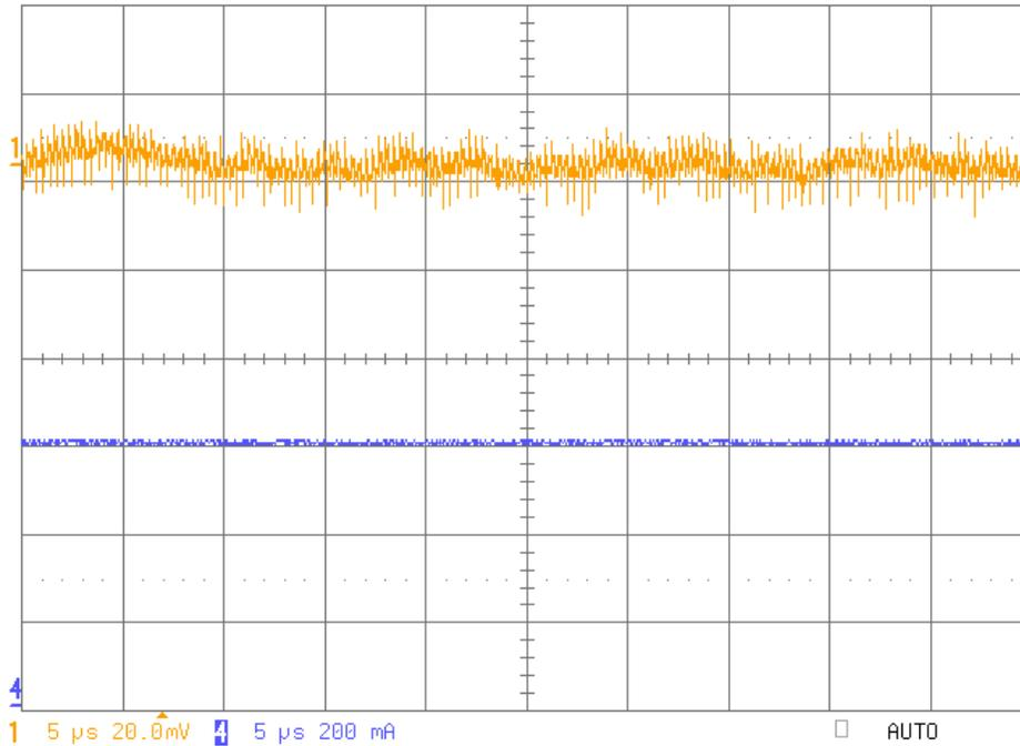
Fig 8: Output Ripple 1.2V (Ch1) @ 0.6A (Ch4) TPS 62353 DCDC, Lowline 3.6V<sub>in</sub>
