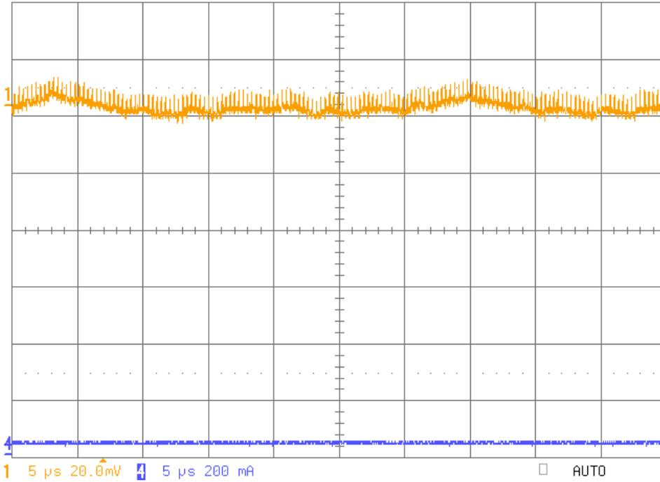
Fig 7: Output Ripple 1.2V (Ch1) @ 0.05A (Ch4) TPS 62353 DCDC, Highline 6V<sub>in</sub>
