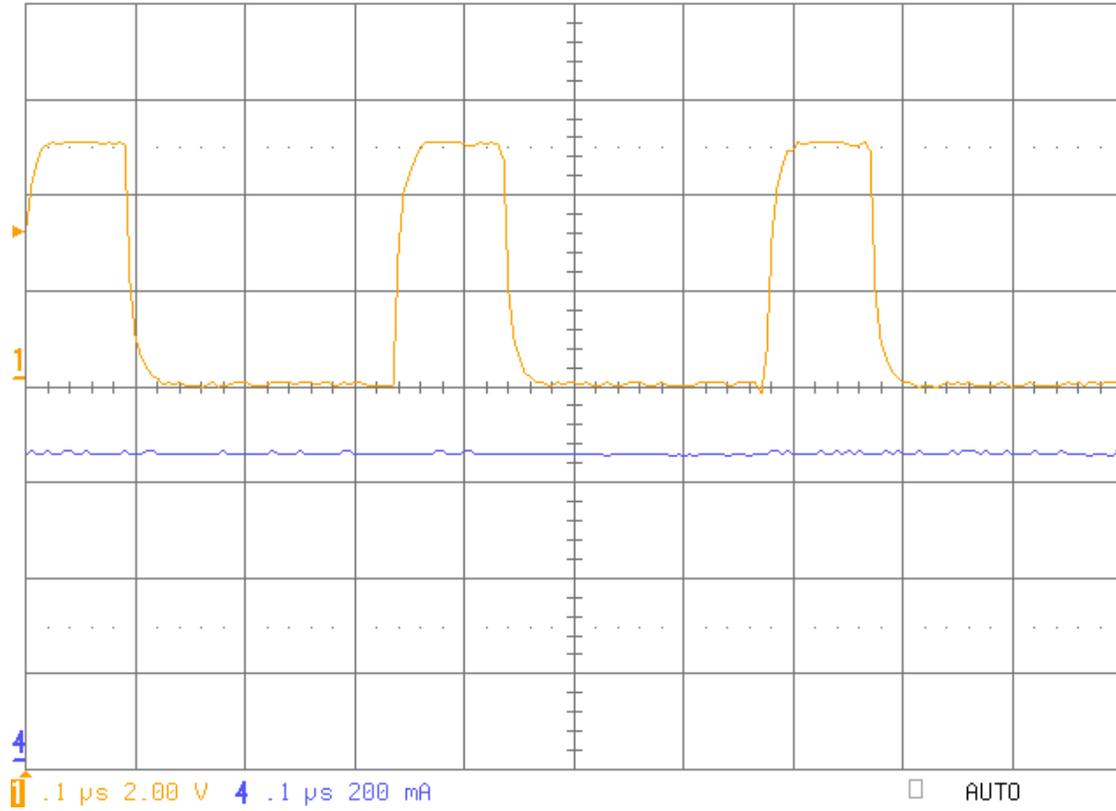
Fig 15: Switch node 1.2V @ 0.6A with 5Vin
