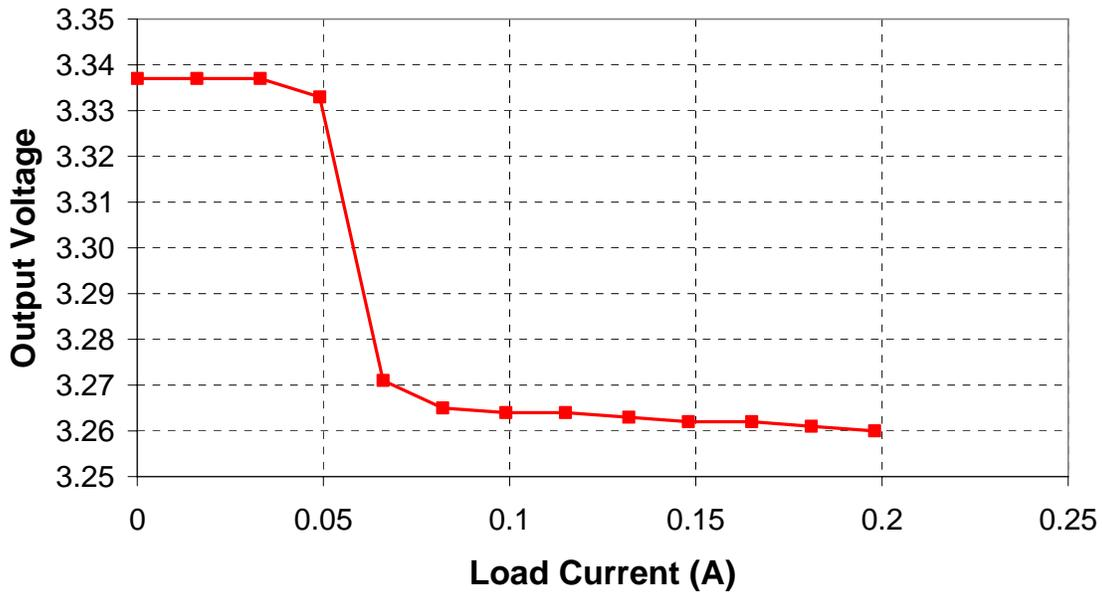
Fig 28: Load Regulation of TPS 62200 5Vin
