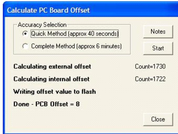
**Figure 1. Board Offset Window in bq208x Evaluation Software**
