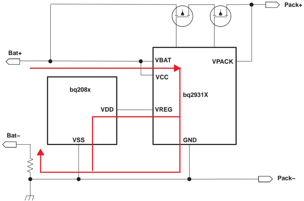
**Figure 2. Measuring Board Offset With Power on Bat+ and Bat- Introduces Error From IC Operation Current**
