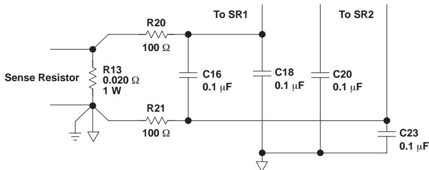
**Figure 5. Recommended Decoupling Circuit for Current Sense Lines**
