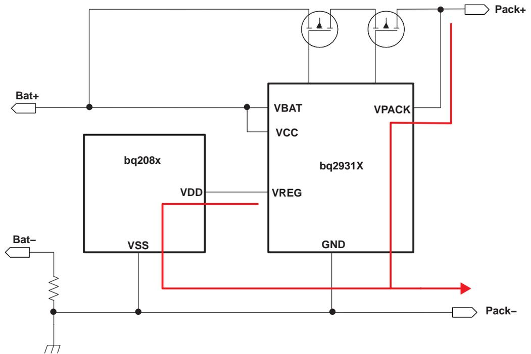
**Figure 3. Powering ICs From Pack+ and Pack- Allows the IC Current to Bypass the Sense Resistor**
