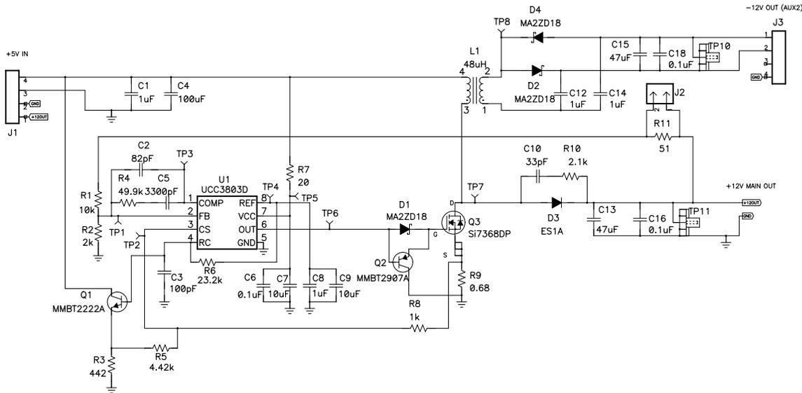
**Figure 3. Boost Converter With Inductively Coupled Auxiliary Output**
