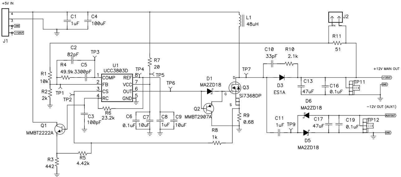
**Figure 2. Boost converter with capacitively coupled auxiliary output.**
