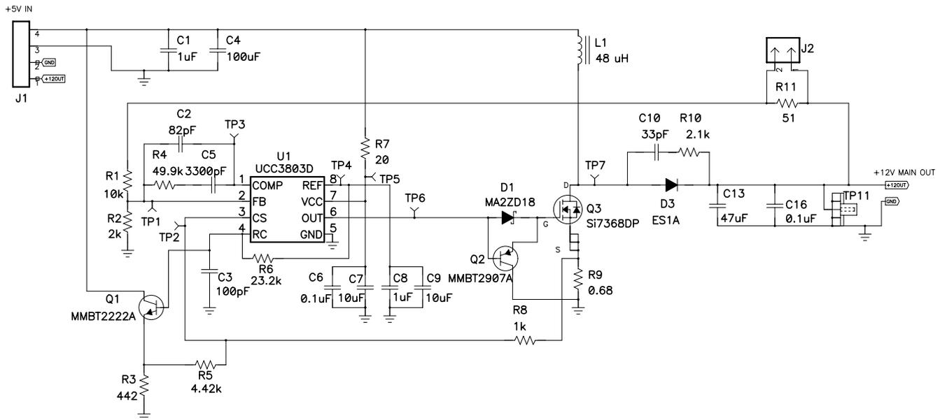
Figure 1. 5-V to 12-V Boost Converter
