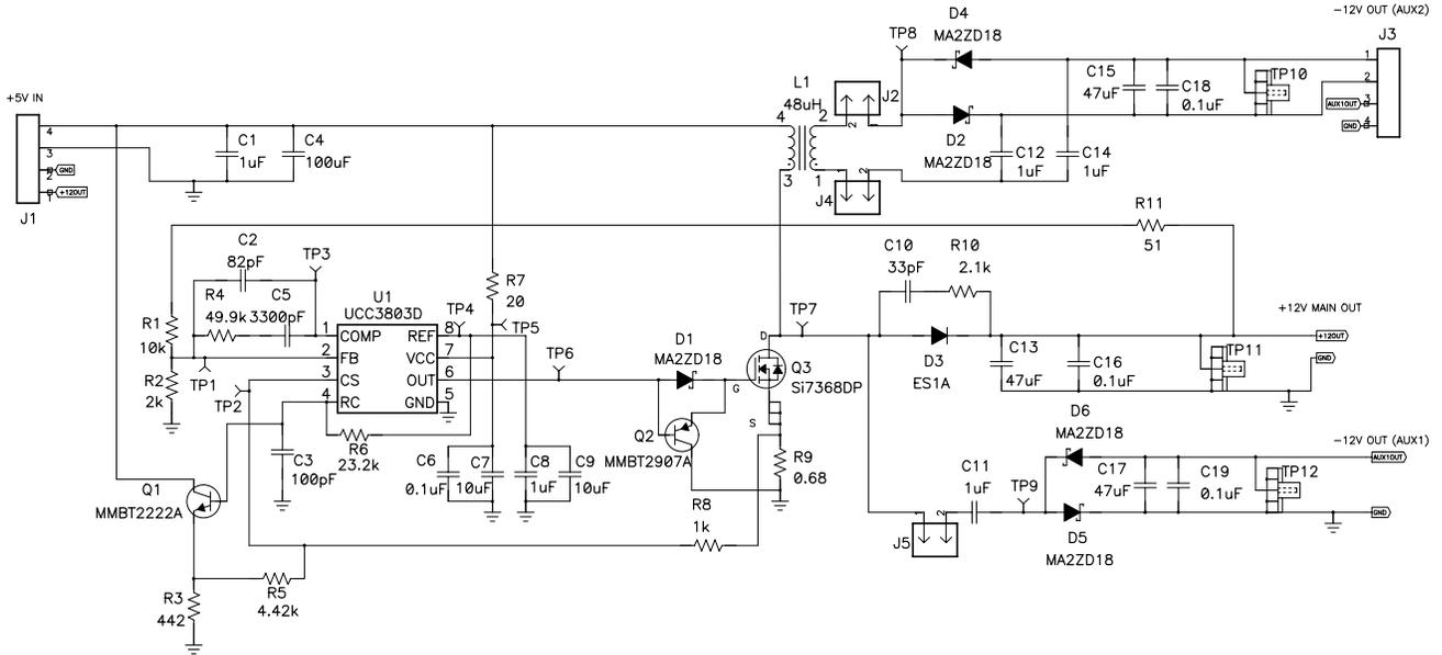
Figure 4. Boost Converter Evaluation Board Containing Both Auxiliary Outputs
