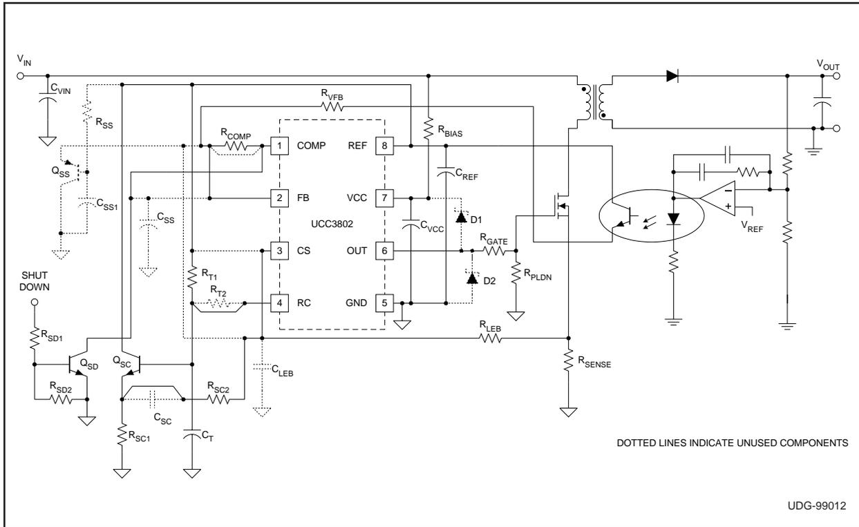
Figure 2. Isolated flyback converter using the UCC3802.
