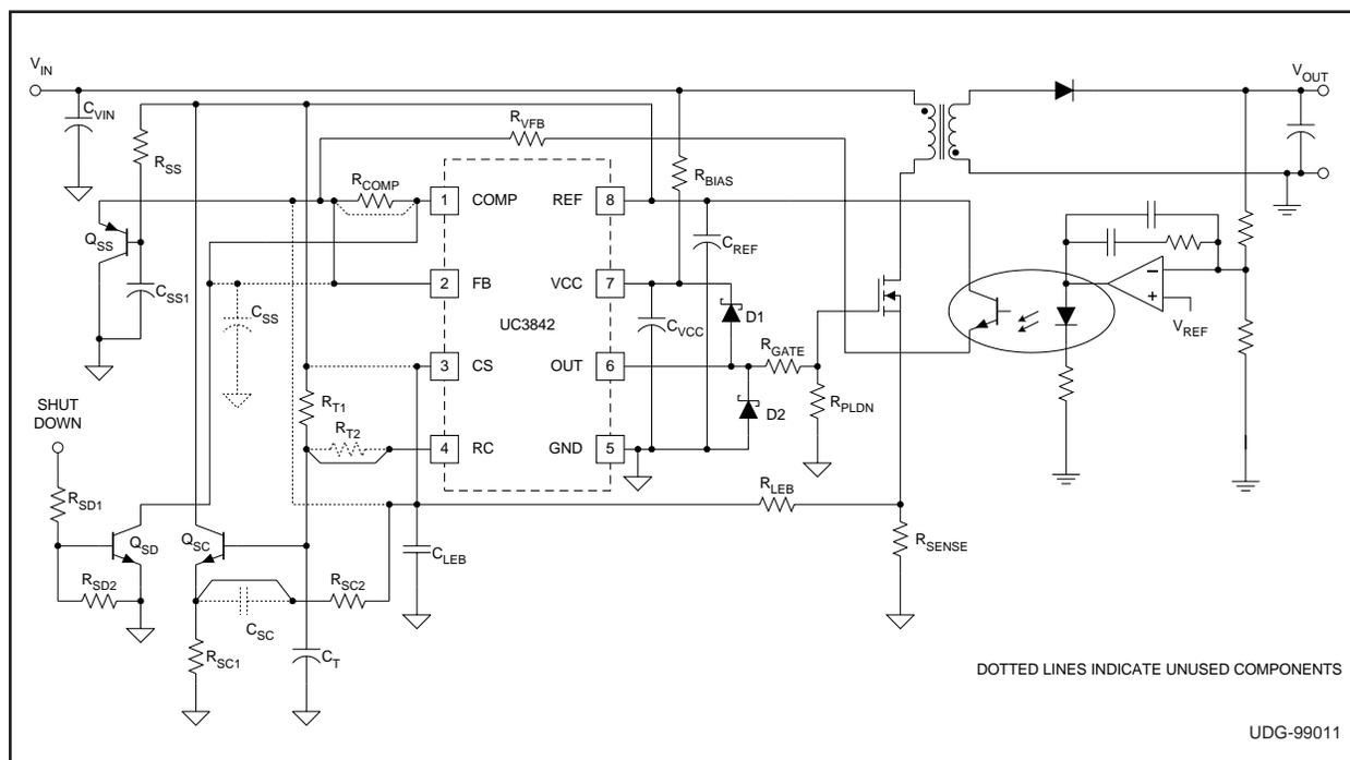
Figure 1. Isolated flyback converter using the UC3842.
