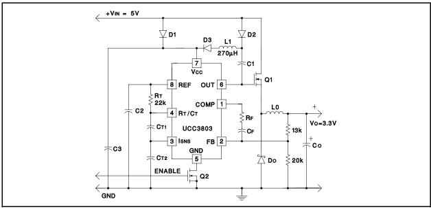
Figure 1. Buck Regulator with High Side NMOS
