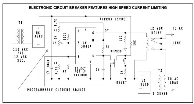
The other input to the PWM comparator is represented by the voltage at pin 1, the error amplifier output which can be adjusted by resistor R2. Internally, this voltage is reduced by two diode drops then attenuated to one-third its amplitude. The PWM circuitry compares this voltage with that of the current sense input at pin 3. When the current sense input exceeds the threshold set by resistor R2, the comparator is tripped and the output at pin 6 is latched OFF.
