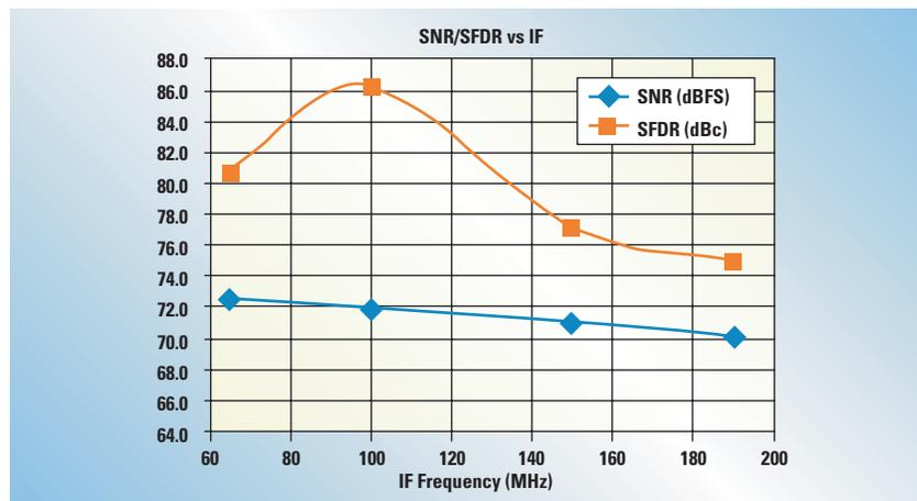
**TSW1000: SNR and SFDR Measurements Clocked at 122.88 MSPS with CDC7005 Plus Amp-BPF**
