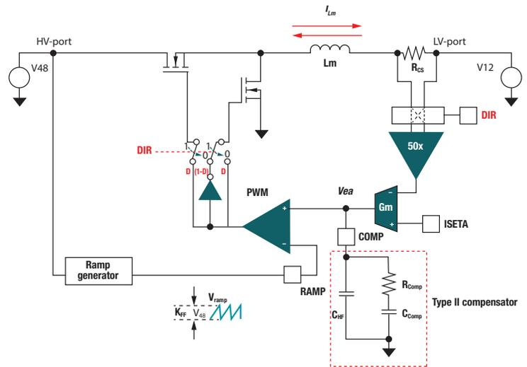
Figure 2. A current control loop of the LM5170.
