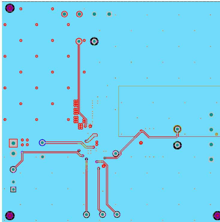
Figure 11. CSD87381PEVM-603 Internal Layer 2 (Top View)
