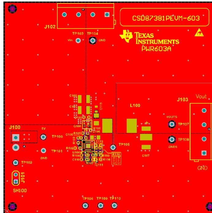
Figure 7. CSD87381PEVM-603 Top Layer Assembly Drawing (Top View)
