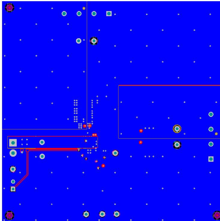
Figure 14. CSD87381PEVM-603 Bottom Copper (Top View)
