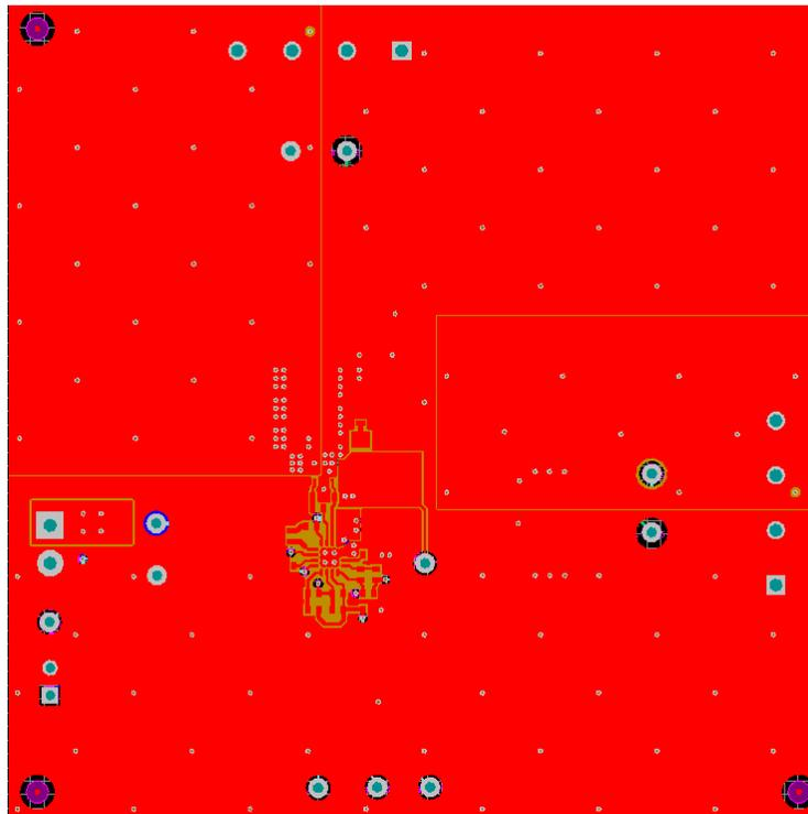
**Figure 9. CSD87381PEVM-603 Top Copper (Top View)**
