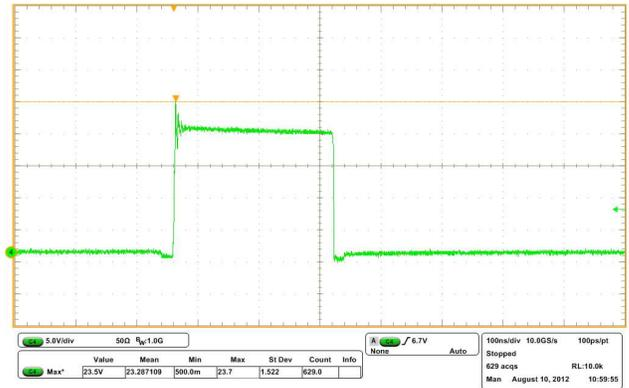
**Figure 6. Switching Node Waveform, VIN = 19 V, Iout = 10 A**
