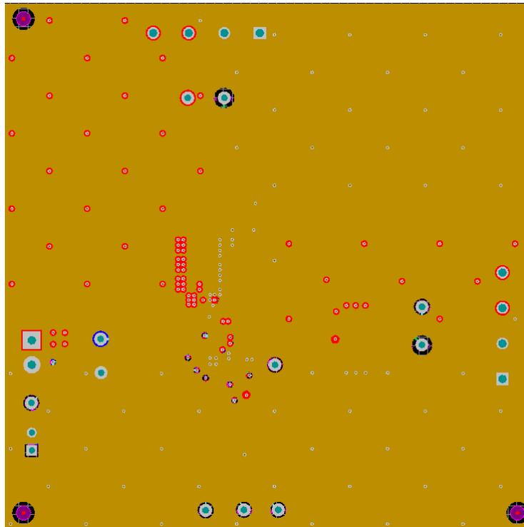
**Figure 10. CSD87381PEVM-603 Internal Layer 1 (Top View)**
