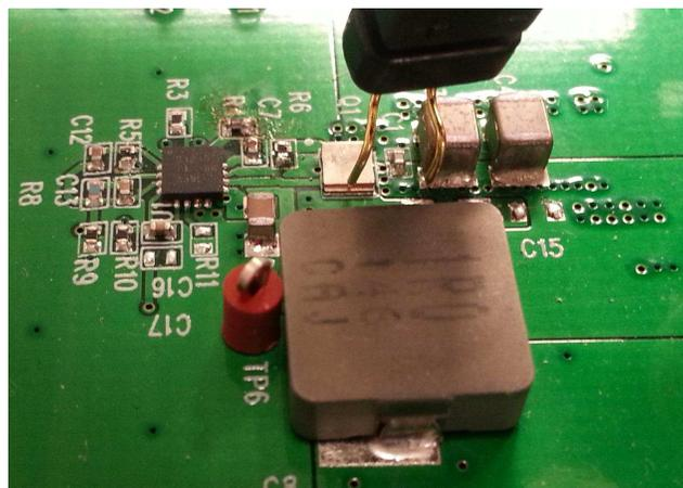
**Figure 2. Tip and Barrel Measurement for Vsw Waveform**
