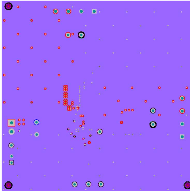
Figure 13. CSD87381PEVM-603 Internal Layer 4 (Top View)
