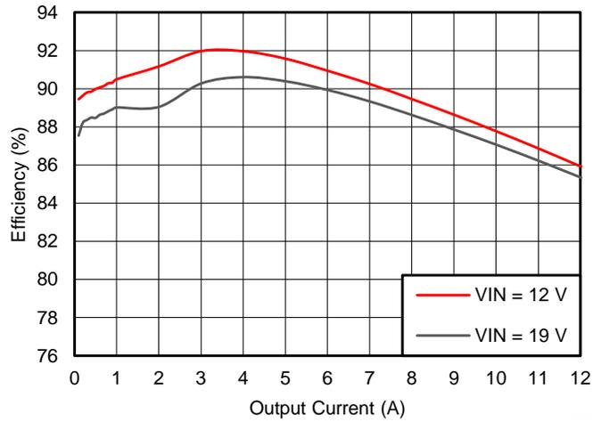
(1) Efficiency at  $V_{GS} = 5.0\text{ V}$ ,  $V_O = 1.35\text{ V}$ ,  $f_{SW} = 300\text{ kHz}$ ,  $L_O = 1\text{ }\mu\text{H}$ ,  $T_A = 25^\circ\text{C}$
