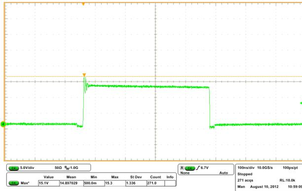
**Figure 5. Switching Node Waveform, VIN = 12 V, Iout = 10 A**
