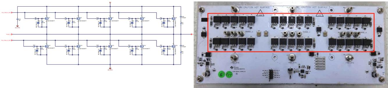
**Figure 5. 5-kW Power-Stage Reference Design Schematic and PCB**
