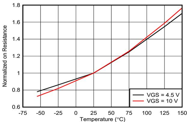
**Figure 1. Power MOSFET On-Resistance vs. Temperature**
